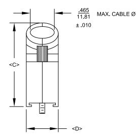
DIMENSIONS(mm/in) \*tolerances are in mm A<sup>+1.70</sup> B<sup>+0.25</sup>  $C_{-0.50}^{+2.40}$ D<sup>+0.85</sup> SIZE 31.00 24.99 36.30 15.00 9 1.220 0.984 1.429 0.591 39.50 33.32 40.30 15.00 15 1.555 1.312 1.587 0.591 53.20 47.04 40.30 15.00 25 1.587 0.591 2.094 1.852 69.70 63.50 40.30 15.00 37 2.744 2.500 1.587 0.591
