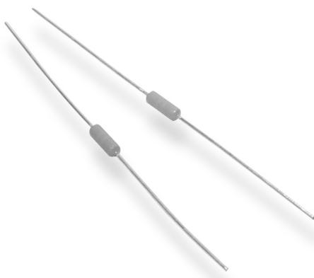
The TE Connectivity Series of Zerohm links are available in two standard case sizes and element types. No end caps are used for the steel element, terminations are welded directly on to the steel slug. For the Ceramic elements, tinned copper wire leads are welded onto end caps. This manufacturing process allows for very low resistance values to be achieved. The slugs are then finished by applying three coats of light brown epoxy resin.
