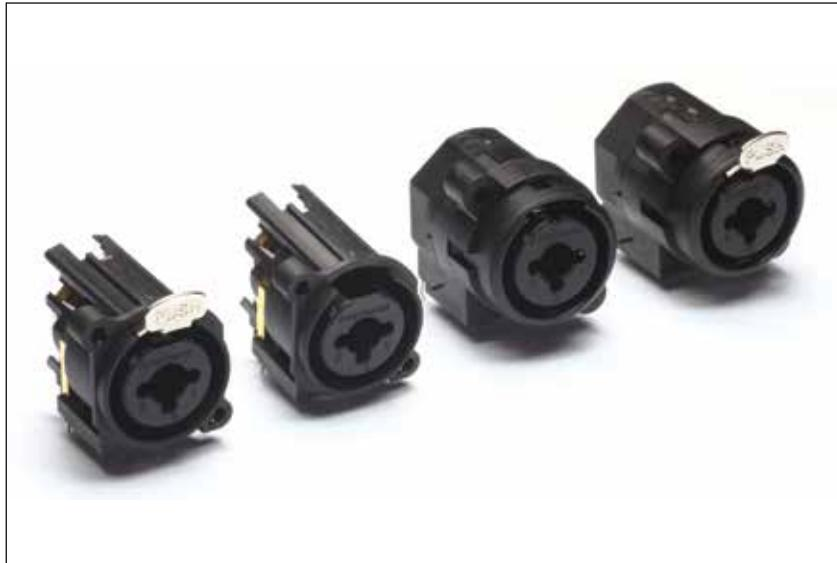
The AC Series C type chassis receptacles feature two connectors in the one space saving housing. A combined XLR female receptacle together with a 6.35mm (1/4") phone jack give the designer more flexibility ensuring premium board space is saved. The new low profile high density C type offers a 15% space saving over the traditional C type. Various configurations are available in either stereo or mono layouts with Vertical, Horizontal Printed Circuit Board or Solder contacts.
