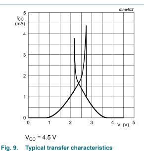
Fig. 8. Typical transfer characteristics
