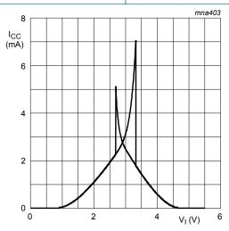
$V_{CC}$  = 5.5 V Fig. 10. Typical transfer characteristics
