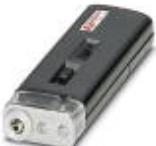
Microscope for visual checks following connector assembly.. 100x zoom, with light. Can be used with two different adapters for F-SMA/B-FOC (ST<sup>®</sup>)/SC-RJ/SC duplex connectors. Dimensions: (L x W x H) 148 x 44 x 23 mm
