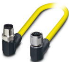
Sensor/actuator cable, 8-position, PVC, yellow, shielded, Plug angled M12 SPEEDCON, coding: A, on Socket angled M12 SPEEDCON, coding: A, cable length: 1.5 m
