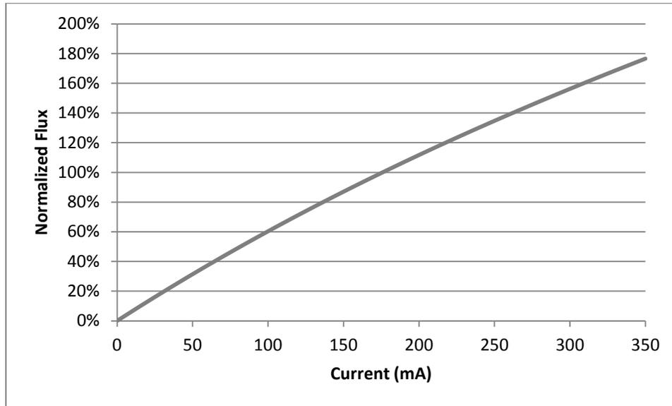
Figure 5: Typical Flux vs. Current – BXRE-xxx-0800-B-xx
