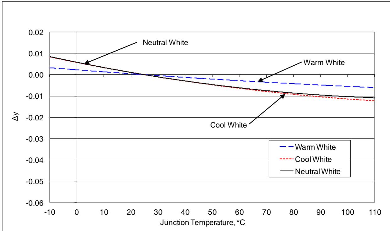
Figure 8: Typical ccx Shift vs. Junction Temperature
