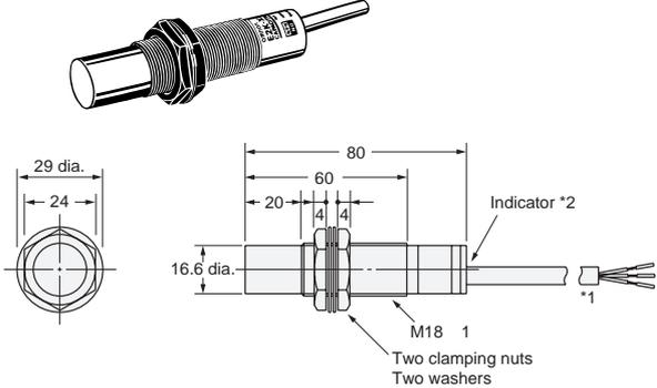
\*1. E and F Models: 6-dia. vinyl-insulated round cable with 3 conductors (Conductor cross section: 0.5 mm<sup>2</sup>, Insulator diameter: 1.9 mm), Standard length: 2 m
