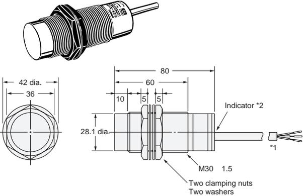
\*1. E and F Models: 6-dia. vinyl-insulated round cable with 3 conductors (Conductor cross section: 0.5 mm<sup>2</sup>, Insulator diameter: 1.9 mm), Standard length: 2 m
