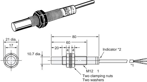
\*1. E and F Models: 4-dia. vinyl-insulated round cable with 3 conductors (Conductor cross section: 0.2 mm<sup>2</sup>, Insulator diameter: 1.2 mm), Standard length: 2 m
