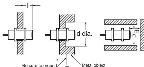
\* Be sure to ground the metal object, otherwise Sensor operation will not be stable.
