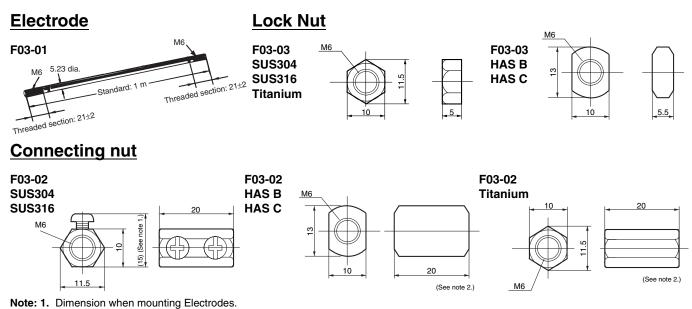
2. Clamp screws are not provided for Hastelloy B, Hastelloy C, or titanium models. F03-03 Lock Nuts are used to mount Electrodes.
