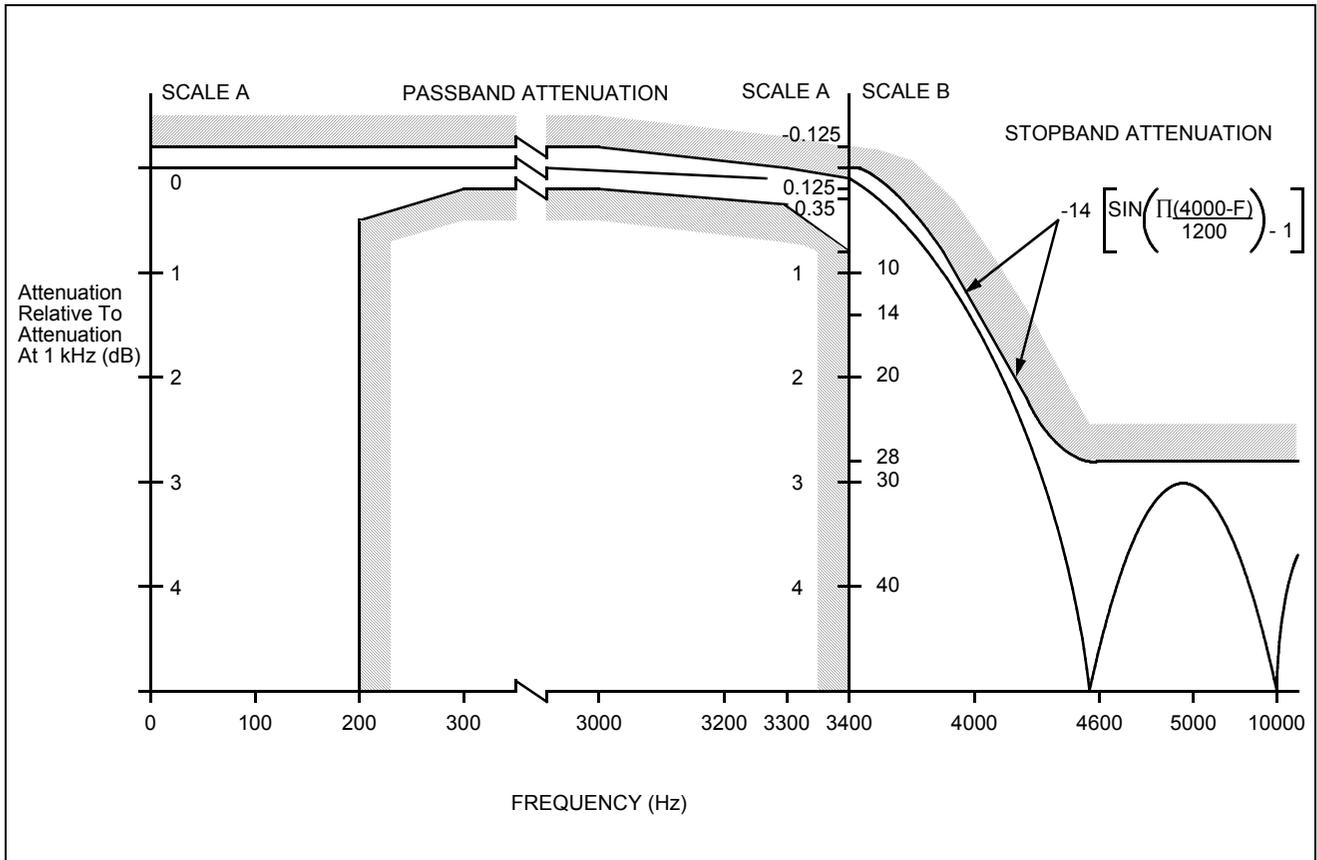
Figure 11 - Attenuation vs Frequency for Receive (D/A) Filter
