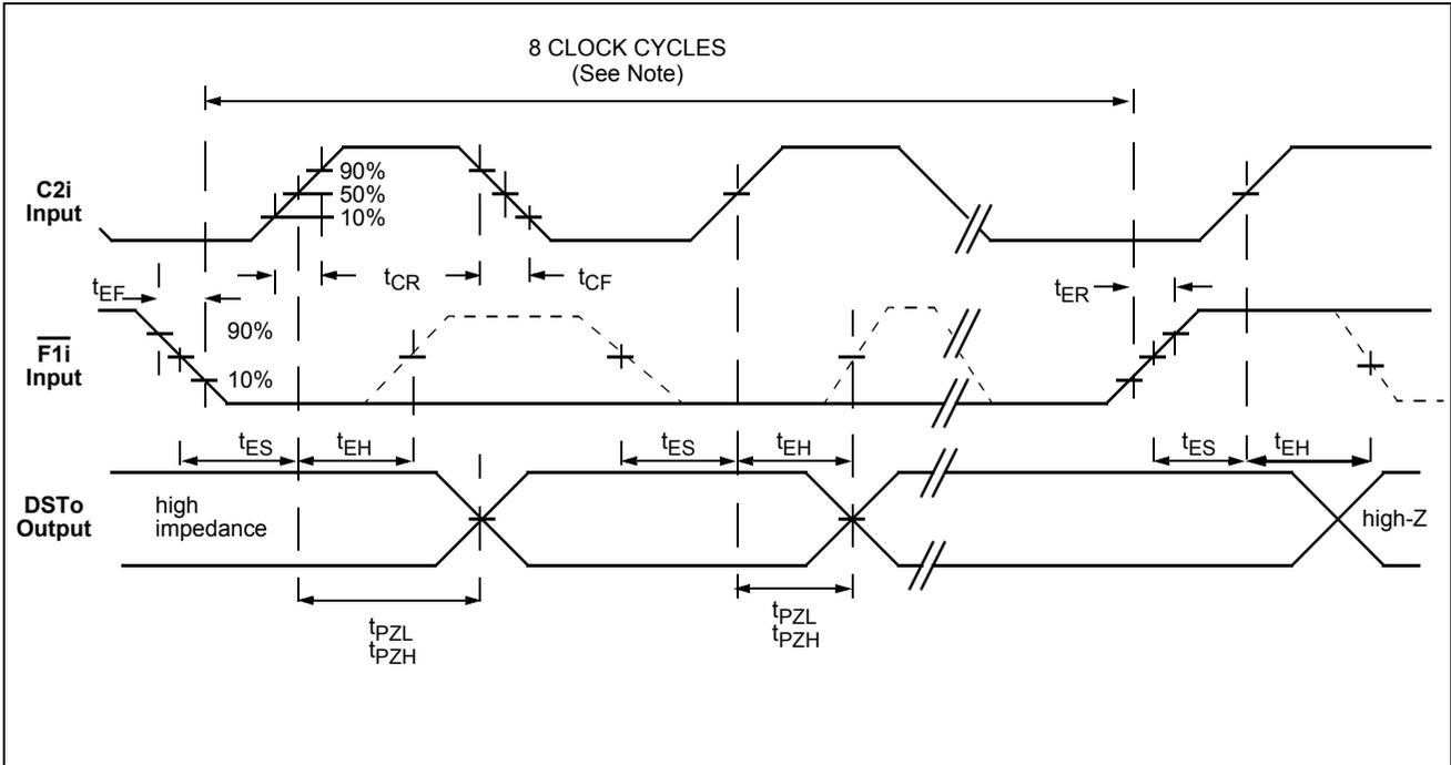
Figure 9b - Timing Diagram - Output Enable
