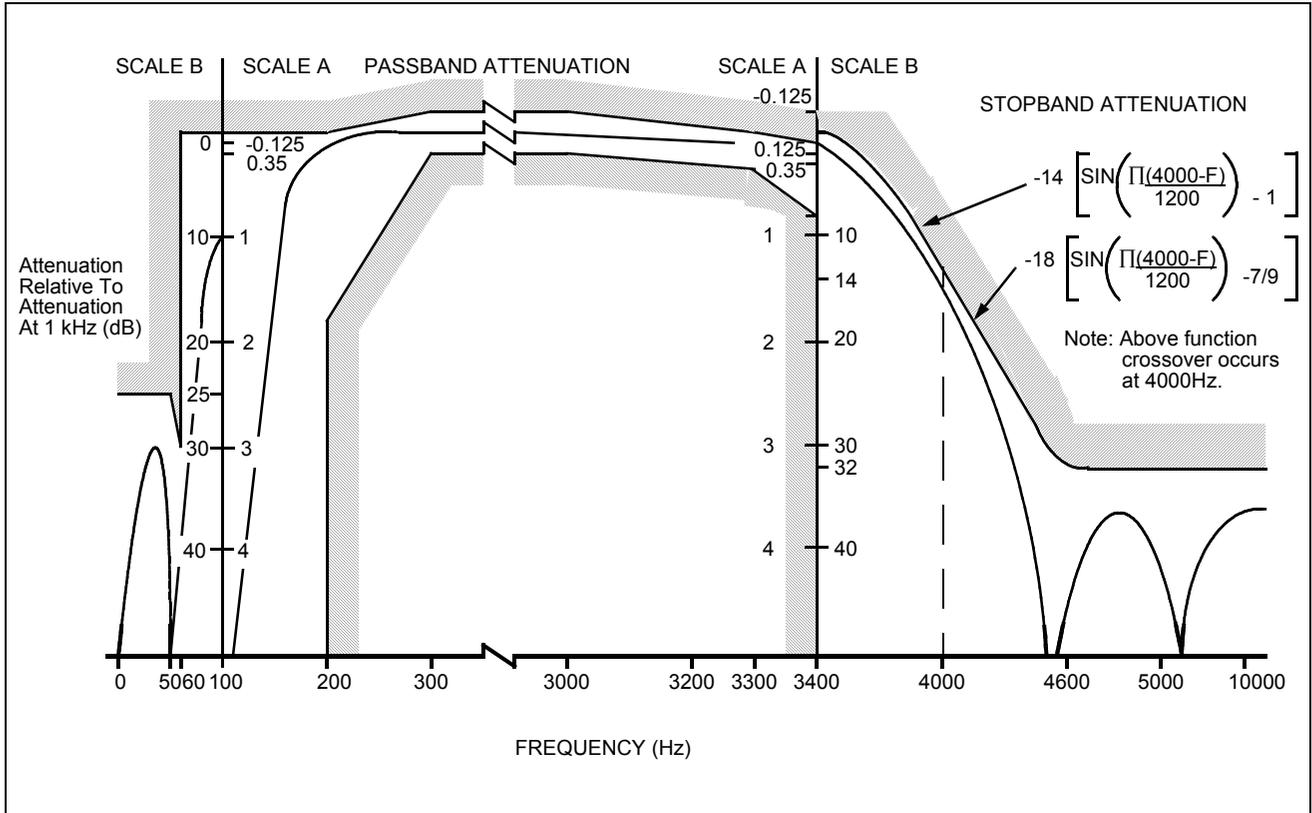
Figure 10 - Attenuation vs Frequency for Transmit (A/D) Filter
