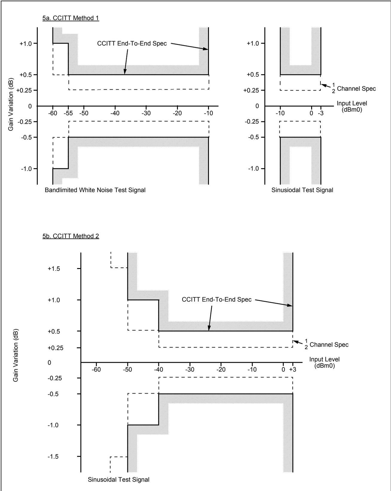
**Figure 12 - Variation of Gain With Input Level**
