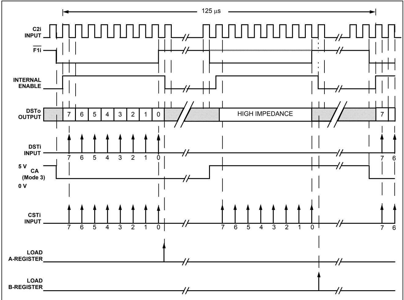
Figure 9a - Timing Diagram - 125 μs Frame Period
