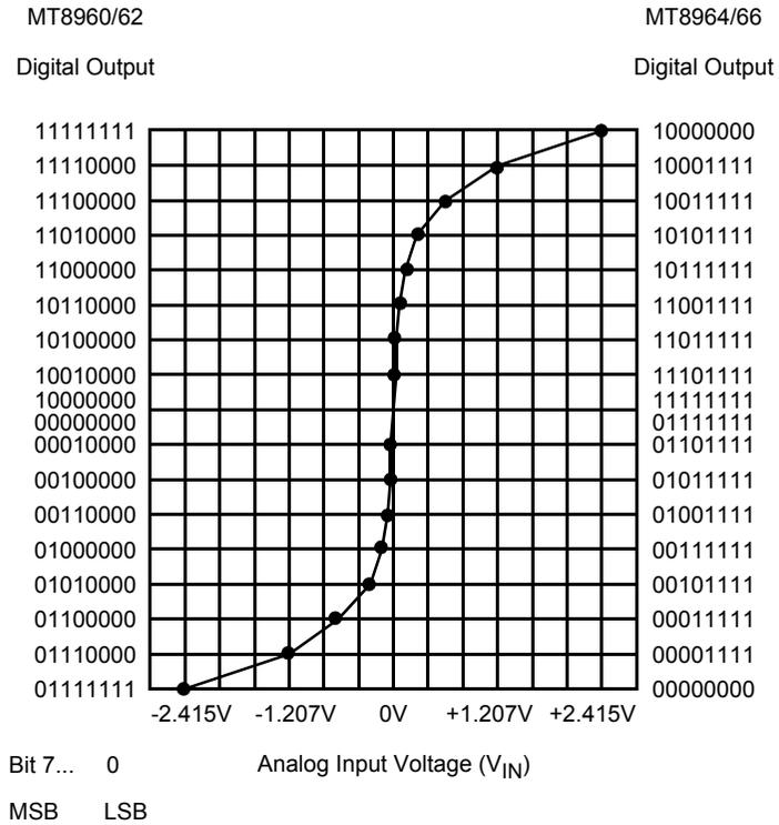
Figure 3 -  $\mu$ -Law Encoder Transfer Characteristic
