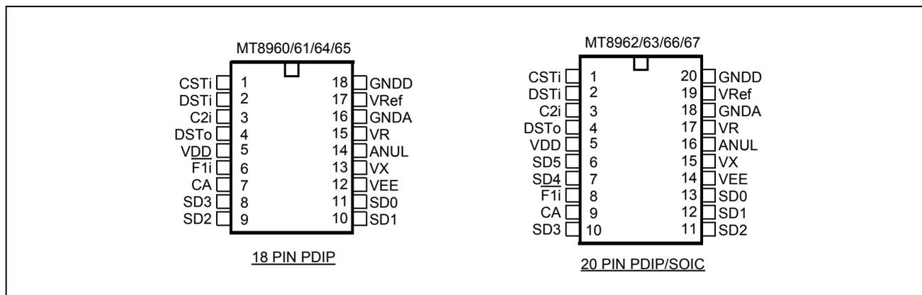
Figure 2 - Pin Connections
