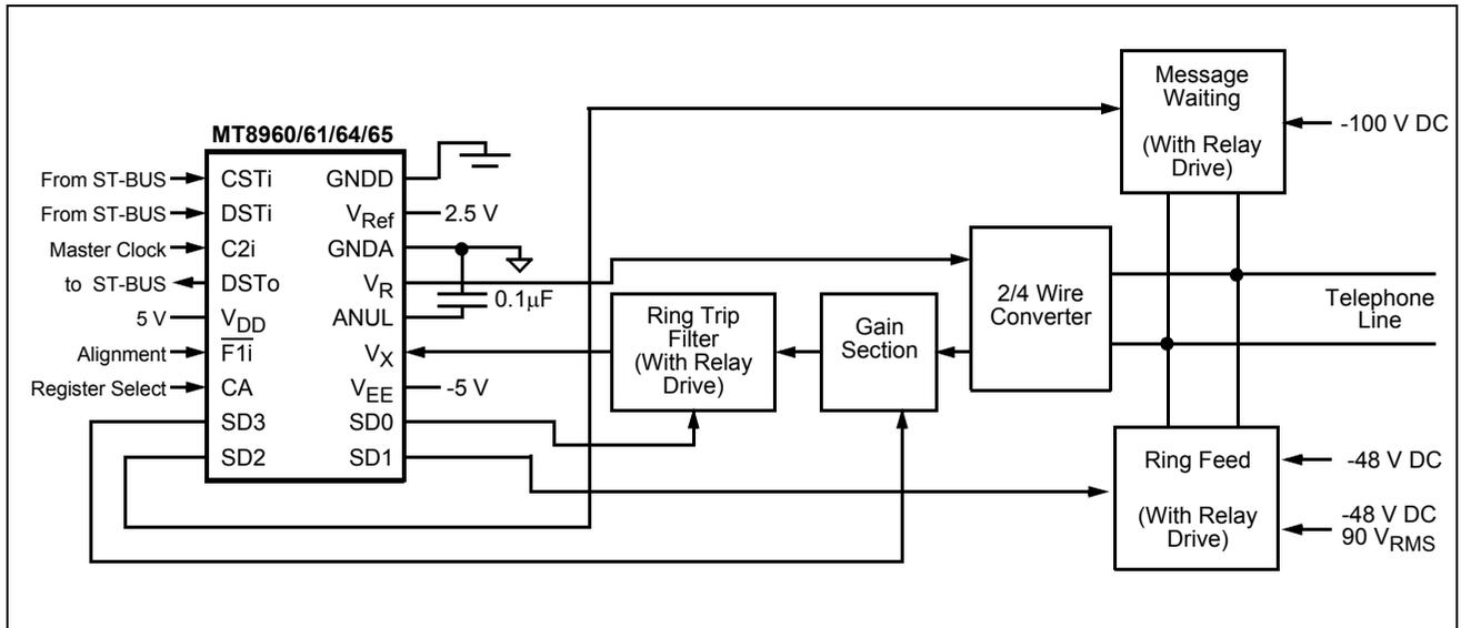
Figure 7 - Typical Use of the Special Drive Outputs
