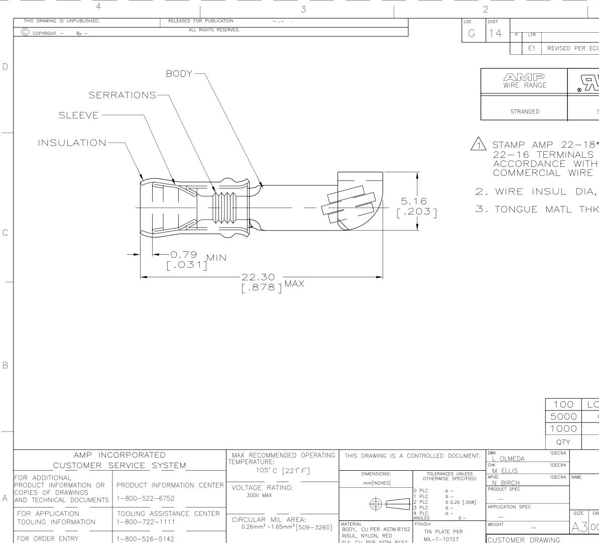
SLV, CU PER ASTM B152
