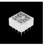
This .150 four pole double throw Grid-space relay is the companion to the two pole 3SBC type shown on page 1-41. It also features the same .150 inch pin spacing that allows you to insert the relay with no intermediate pin spreaders. There is adequate clearance for conductors to reach all pins. It is a very compact 4 pole double throw 2 ampere relay.
