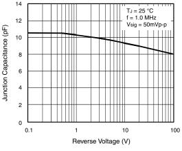
Fig. 5 - Typical Junction Capacitance
