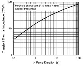
Fig. 6 - Typical Thermal Impedance
