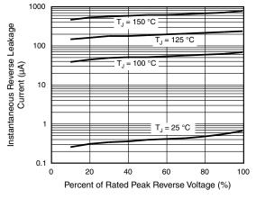
Fig. 4 - Typical Reverse Leakage Characteristics
