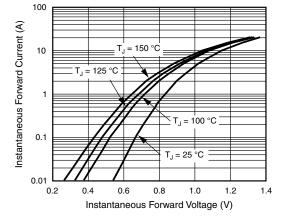
Fig. 3 - Typical Instantaneous Forward Characteristics
