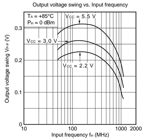
Divide by 4 mode (Guaranteed operating window:  $V_{CC} = 2.2$  to  $5.5$  V,  $T_A = -40$  to  $+85^\circ\text{C}$ )
