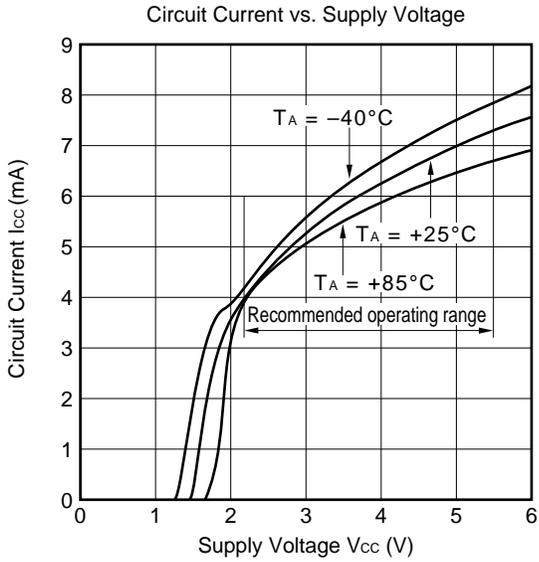
Divide by 2 mode (Guaranteed operating window:  $V_{CC} = 2.2$  to  $5.5$  V,  $T_A = -40$  to  $+85^\circ\text{C}$ )
