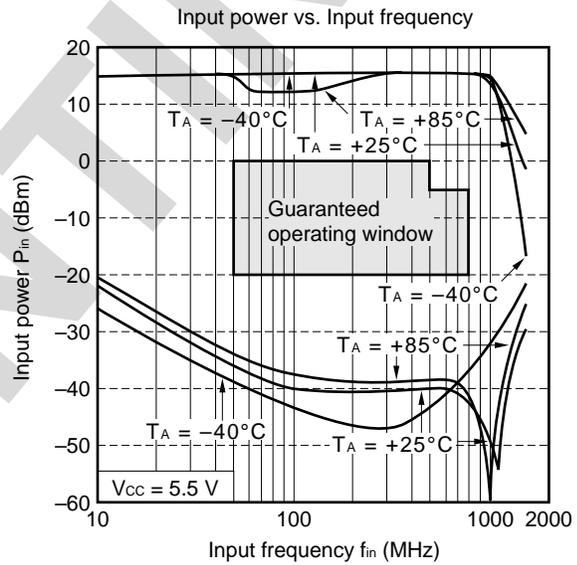
Divide by 8 mode (Guaranteed operating window:  $V_{CC} = 2.2$  to  $5.5$  V,  $T_A = -40$  to  $+85^\circ\text{C}$ )
