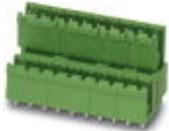
Header, Nominal current: 10 A, Rated voltage (III/2): 320 V, Number of positions: 8, Pitch: 5 mm, Color: green, Contact surface: Tin, Mounting: Wave soldering, Can be aligned! Mounting flange: Order No. 1836477, 1836480. In combination with MVSTB or FKCV plug components, both an MVSTBW (or FKCVW) and an MVSTBR plug (or FKCVR) must be used. Combination with TMSTBP plug components is not possible!
