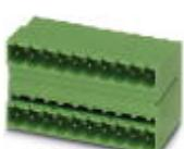
Header, Nominal current: 10 A, Rated voltage (III/2): 320 V, Number of positions: 8, Pitch: 5 mm, Color: green, Contact surface: Tin, Mounting: Wave soldering, In combination with MVSTB or FKCV plug components, both an MVSTBW (or FKCVW) and an MVSTBR plug (or FKCVR) must be used. Combination with TMSTBP plug components is not possible!
