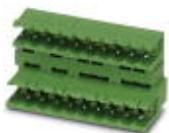
Header, Nominal current: 10 A, Rated voltage (III/2): 320 V, Number of positions: 8, Pitch: 5 mm, Color: green, Contact surface: Tin, Mounting: Wave soldering, Can be aligned! Mounting flange: Order No. 1736771, 1736768. In combination with MVSTB or FKCV plug components, both an MVSTBW (or FKCVW) and an MVSTBR plug (or FKCVR) must be used. Combination with TMSTBP plug components is not possible!
