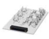
Header, Nominal current: 12 A, Rated voltage (III/2): 320 V, Number of positions: 8, Pitch: 5 mm, Color: black, Contact surface: Tin, Mounting: Soldering, User information and design recommendations for through hole reflow technology can be found under "Downloads"
