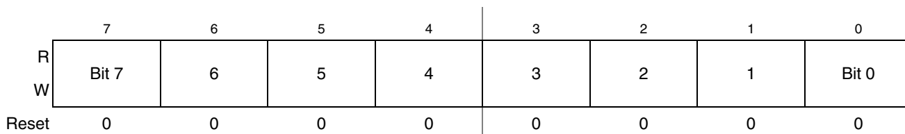
Figure 15-14. TPM Channel Value Register Low (TPMxCnVL)
