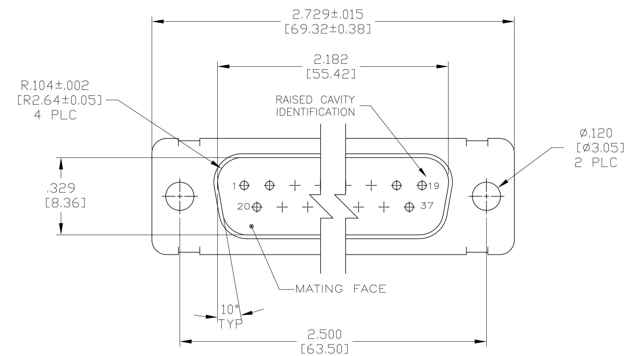
1. THIS CONNECTOR ASSEMBLY IS SUPPLIED WITH Be Cu CONTACT RETENTION CLIPS INSTALLED IN THE INSERT ASSEMBLY.
