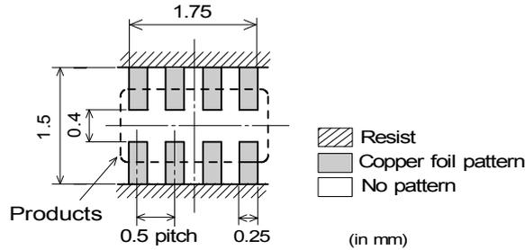
**16.7 Standard Soldering Condition (Reflow soldering)**
