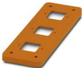
Adapter plates, with reinforced wall, 3 cutouts for connectors HC-D 7, cutout 3 x 21.5 x 21.5, for type B24 to D7
