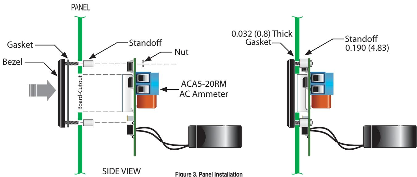
Figure 3. Panel Installation
