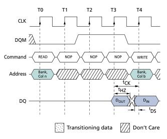
Note: 1. CL = 3. The READ command can be issued to any bank, and the WRITE command can be to any bank. If a burst of one is used, DQM is not required.
