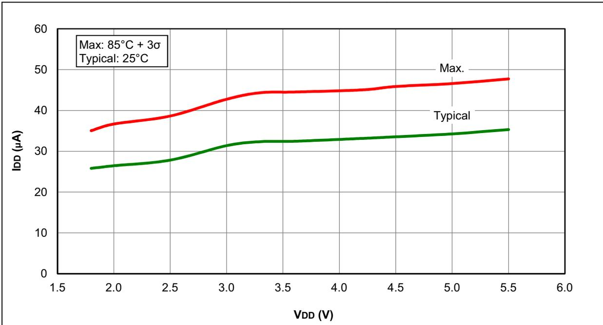
**FIGURE 31-3: I<sub>DD</sub> TYPICAL, XT AND EXTRC OSCILLATOR MODE, PIC16LF1933 ONLY**
