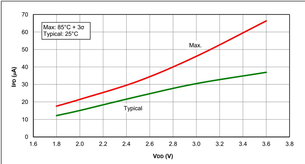
**FIGURE 31-44: I<sub>PD</sub>, CAPACITIVE SENSING (CPS) MODULE, HIGH-CURRENT RANGE, CPSRM = 0, CPSRNG = 11, PIC16F1933 ONLY**
