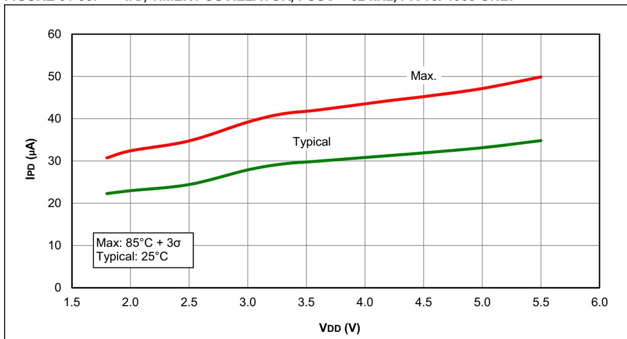
**FIGURE 31-39: I<sub>PD</sub>, CAPACITIVE SENSING (CPS) MODULE, LOW-CURRENT RANGE, CPSRM = 0, CPSRNG = 01, PIC16LF1933 ONLY**
