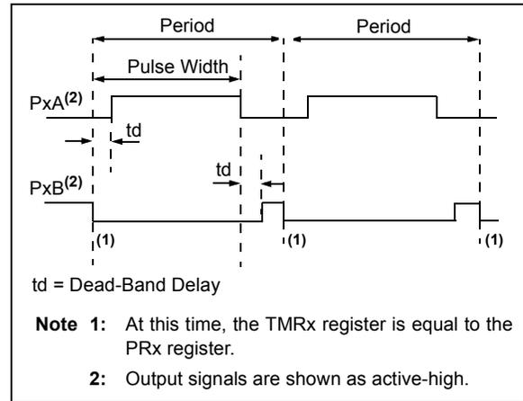
**FIGURE 23-9: EXAMPLE OF HALF-BRIDGE APPLICATIONS**
