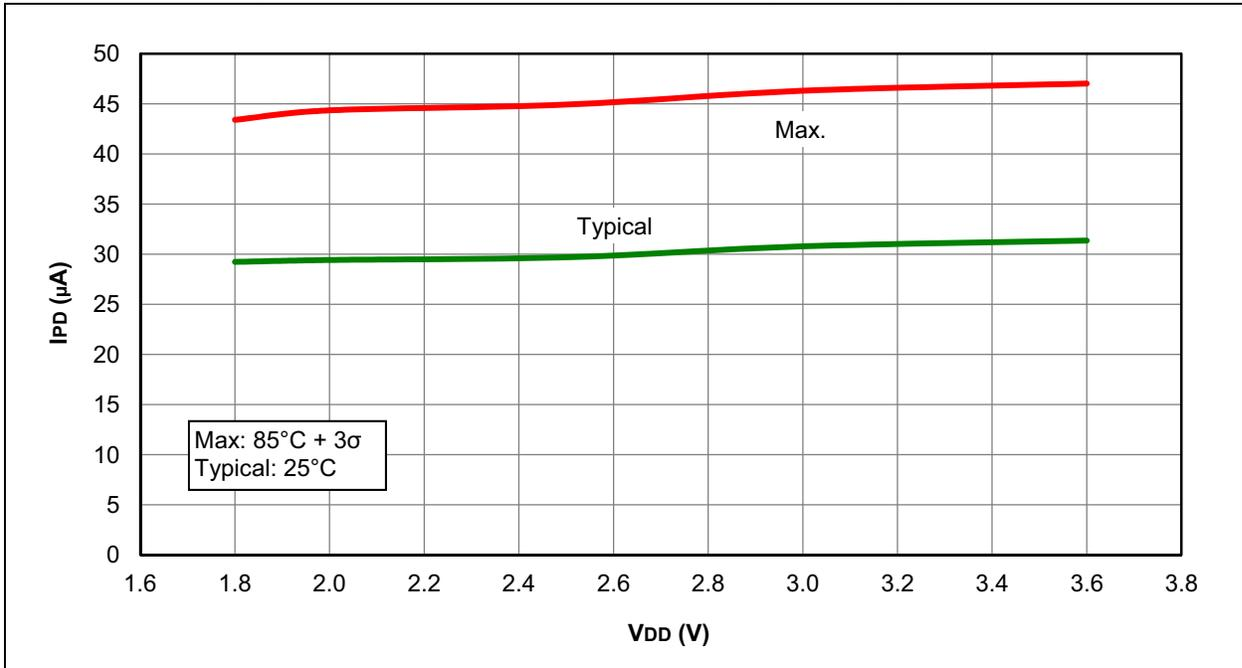
FIGURE 31-48: I<sub>PD</sub>, COMPARATOR, NORMAL-POWER MODE, C<sub>xSP</sub> = 1, PIC16F1933 ONLY
