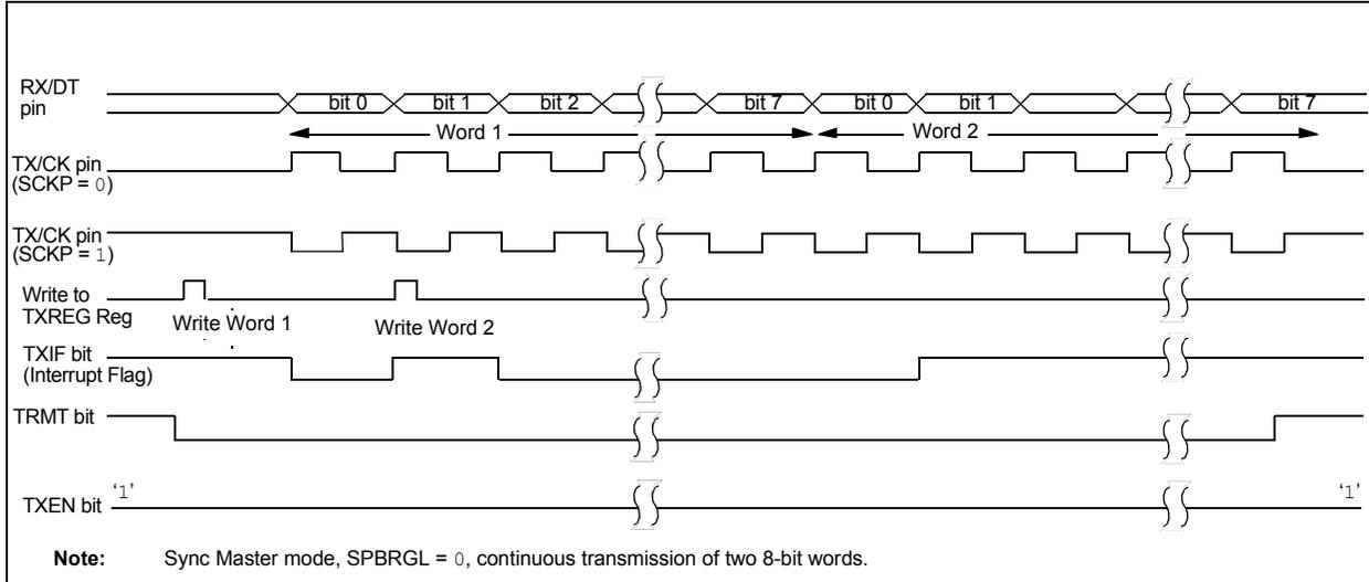
**FIGURE 25-11: SYNCHRONOUS TRANSMISSION (THROUGH TXEN)**
