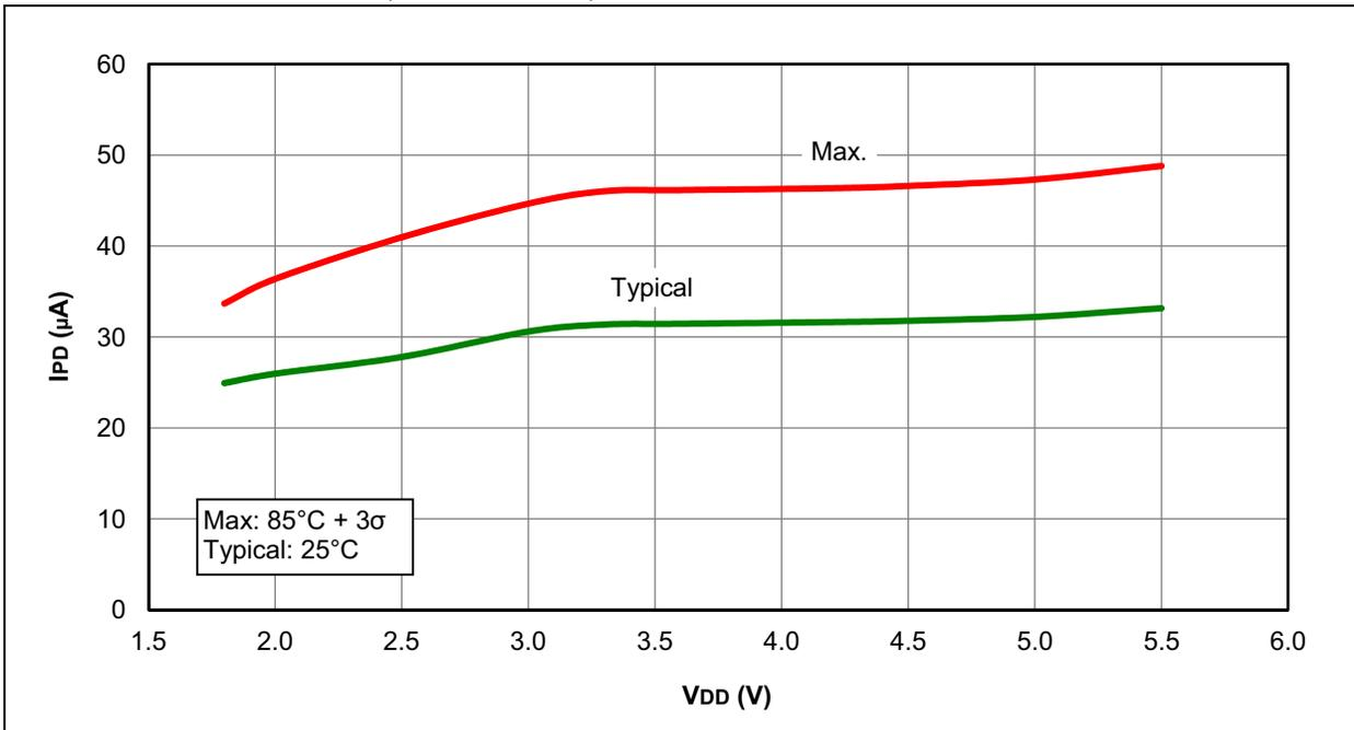
**FIGURE 31-43: I<sub>PD</sub>, CAPACITIVE SENSING (CPS) MODULE, HIGH-CURRENT RANGE, CPSRM = 0, CPSRNG = 11, PIC16LF1933 ONLY**
