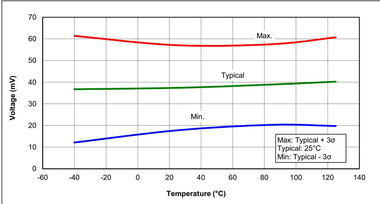
**FIGURE 31-59: BROWN-OUT RESET VOLTAGE, BORV = 0**
