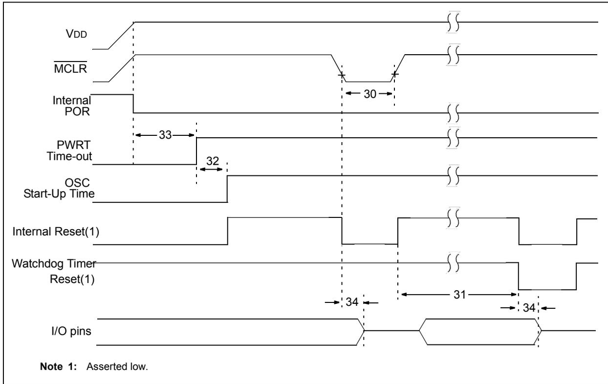
**FIGURE 30-9: BROWN-OUT RESET TIMING AND CHARACTERISTICS**
