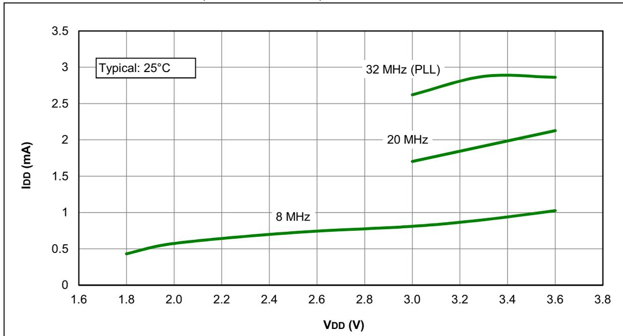
FIGURE 31-26: I<sub>DD</sub> MAXIMUM, HS OSCILLATOR, PIC16LF1933 ONLY
