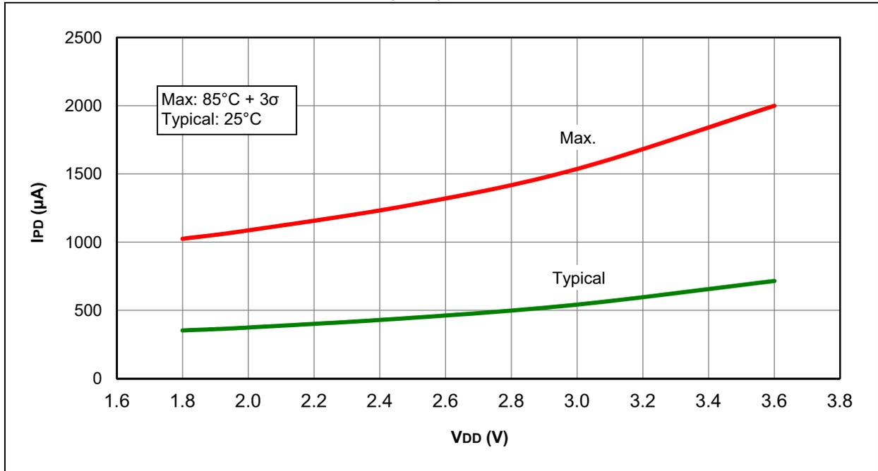
**FIGURE 31-32: I<sub>PD</sub>, WATCHDOG TIMER (WDT), PIC16F1933 ONLY**
