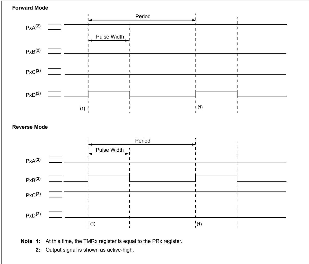
**FIGURE 23-13: EXAMPLE OF PWM DIRECTION CHANGE AT NEAR 100% DUTY CYCLE**
