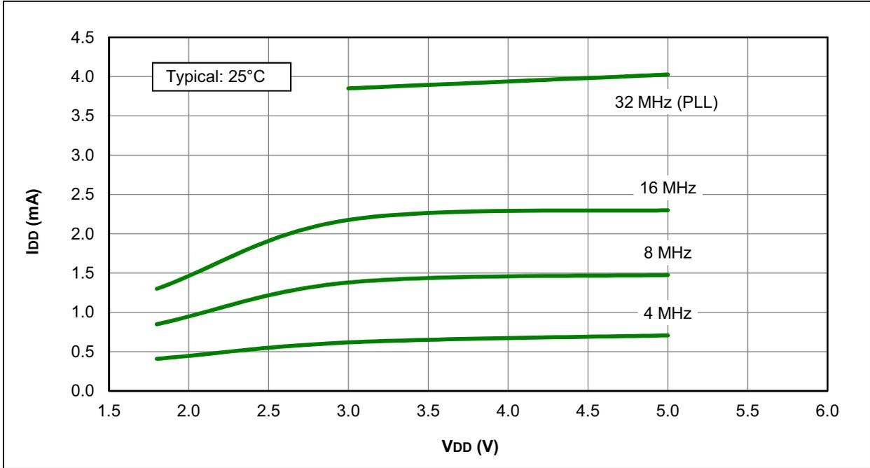
**FIGURE 31-24: I<sub>DD</sub> MAXIMUM, HFINTOSC MODE, PIC16F1933 ONLY**
