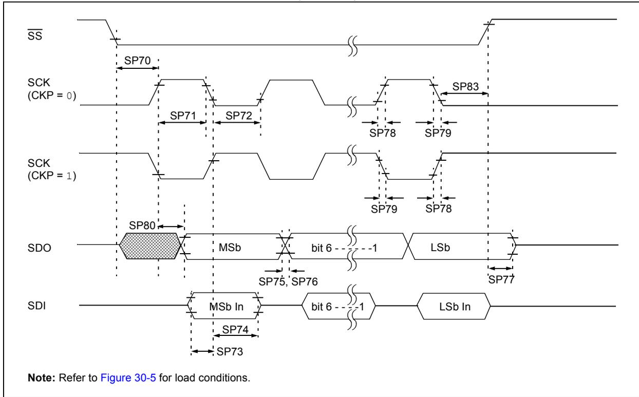
**FIGURE 30-19: SPI SLAVE MODE TIMING (CKE = 1)**
