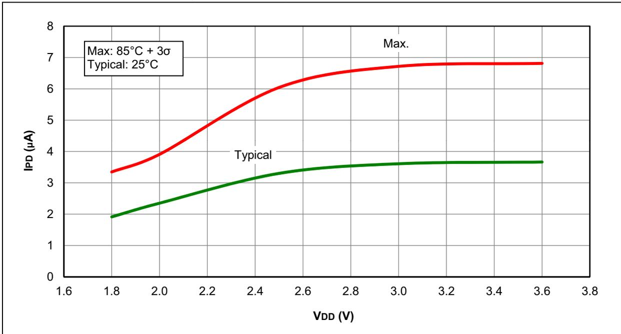
**FIGURE 31-40: I<sub>PD</sub>, CAPACITIVE SENSING (CPS) MODULE, LOW-CURRENT RANGE, CPSRM = 0, CPSRNG = 01, PIC16F1933 ONLY**
