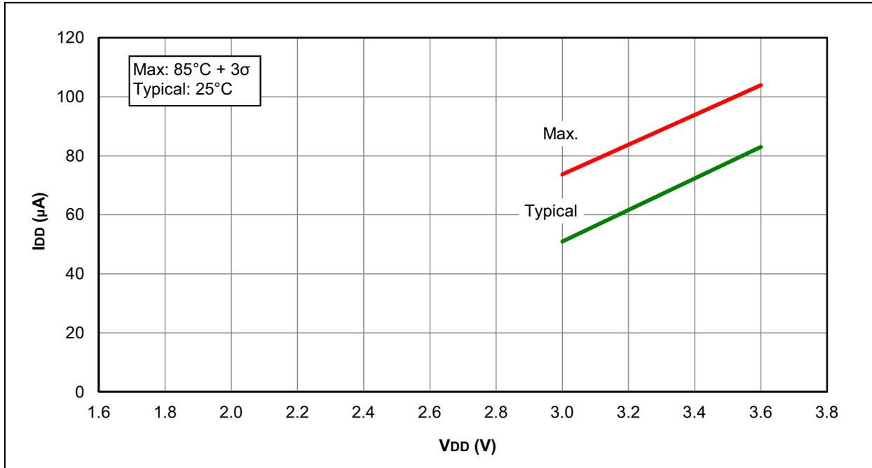
**FIGURE 31-8: I<sub>DD</sub>, EC OSCILLATOR, LOW-POWER MODE, FOSC = 500 kHz, PIC16F1933 ONLY**
