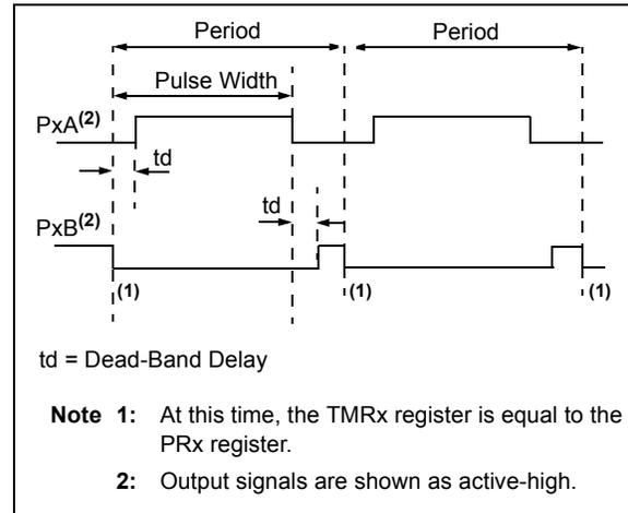
**FIGURE 23-17: EXAMPLE OF HALF-BRIDGE APPLICATIONS**
