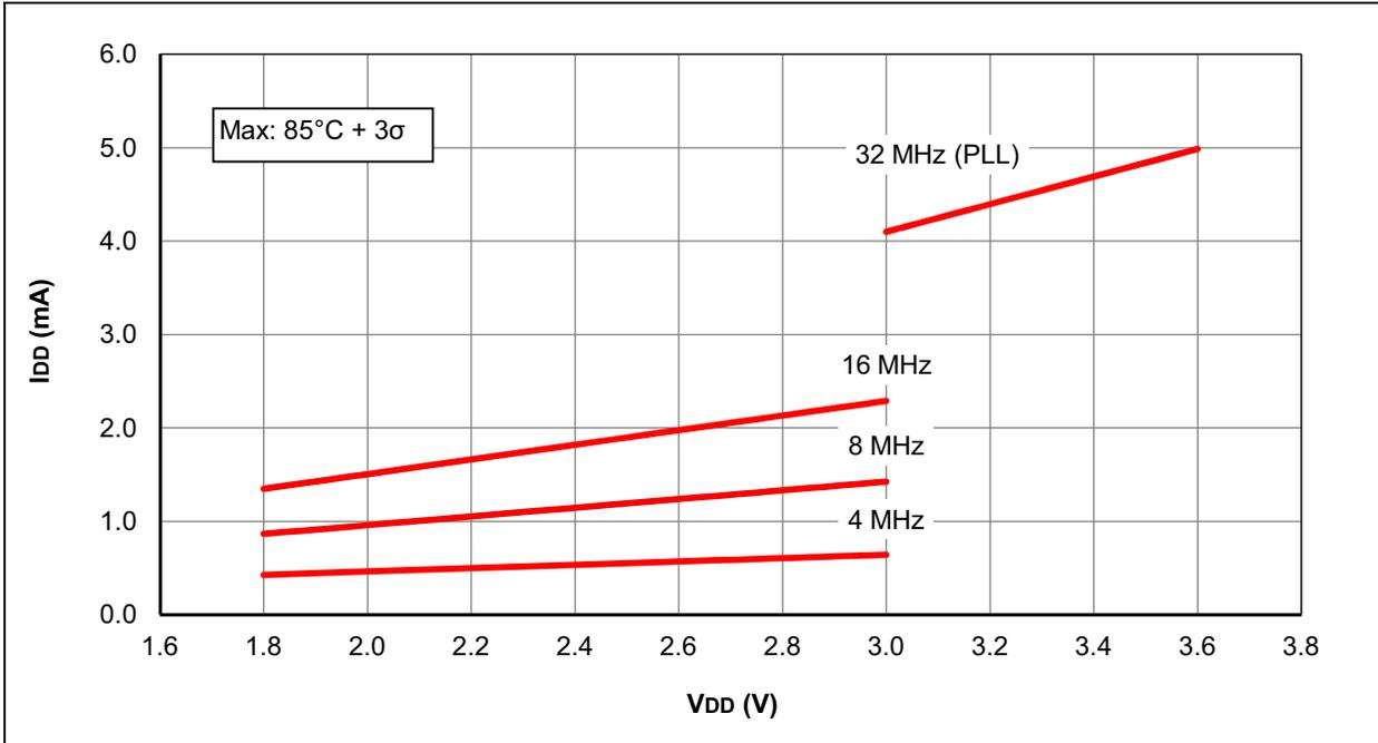
**FIGURE 31-23: I<sub>DD</sub> TYPICAL, HFINTOSC MODE, PIC16F1933 ONLY**
