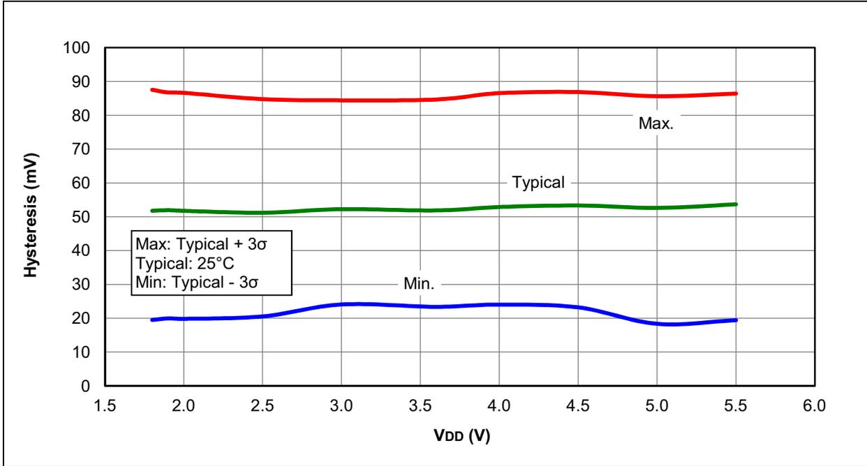
FIGURE 31-64: COMPARATOR HYSTERESIS, LOW-POWER MODE, CxSP = 0, CxHYS = 1
