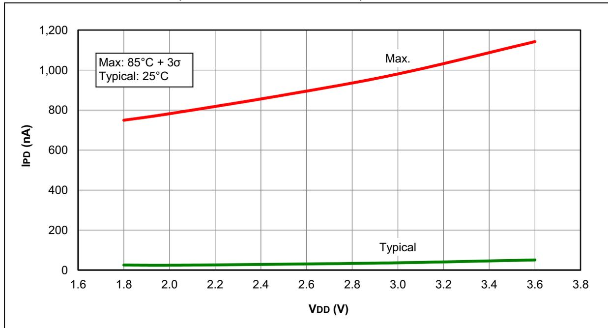
FIGURE 31-30: I<sub>PD</sub> BASE, LOW-POWER SLEEP MODE, PIC16F1933 ONLY
