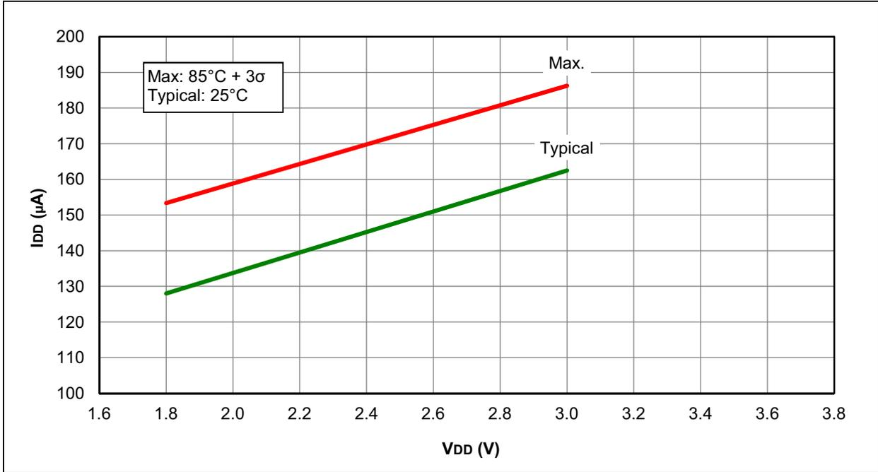
**FIGURE 31-20: I<sub>DD</sub>, MFINTOSC MODE, FOSC = 500 kHz, PIC16F1933 ONLY**
