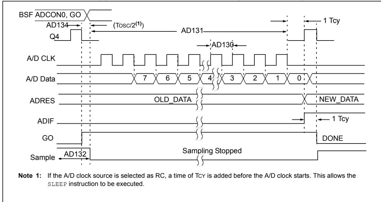
**FIGURE 30-13: PIC16(L)F1933 A/D CONVERSION TIMING (SLEEP MODE)**
