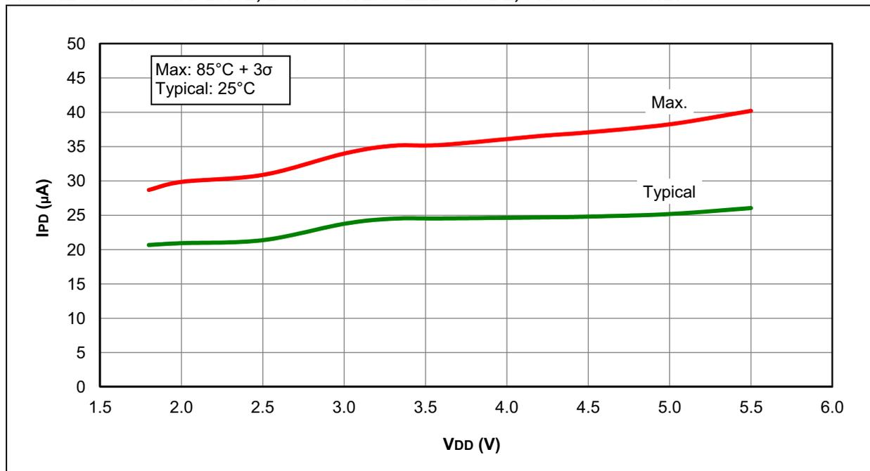
**FIGURE 31-31: I<sub>PD</sub>, WATCHDOG TIMER (WDT), PIC16LF1933 ONLY**
