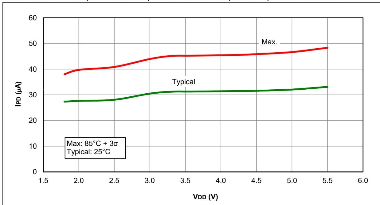
FIGURE 31-47: I<sub>PD</sub>, COMPARATOR, NORMAL-POWER MODE, C<sub>xSP</sub> = 1, PIC16LF1933 ONLY
