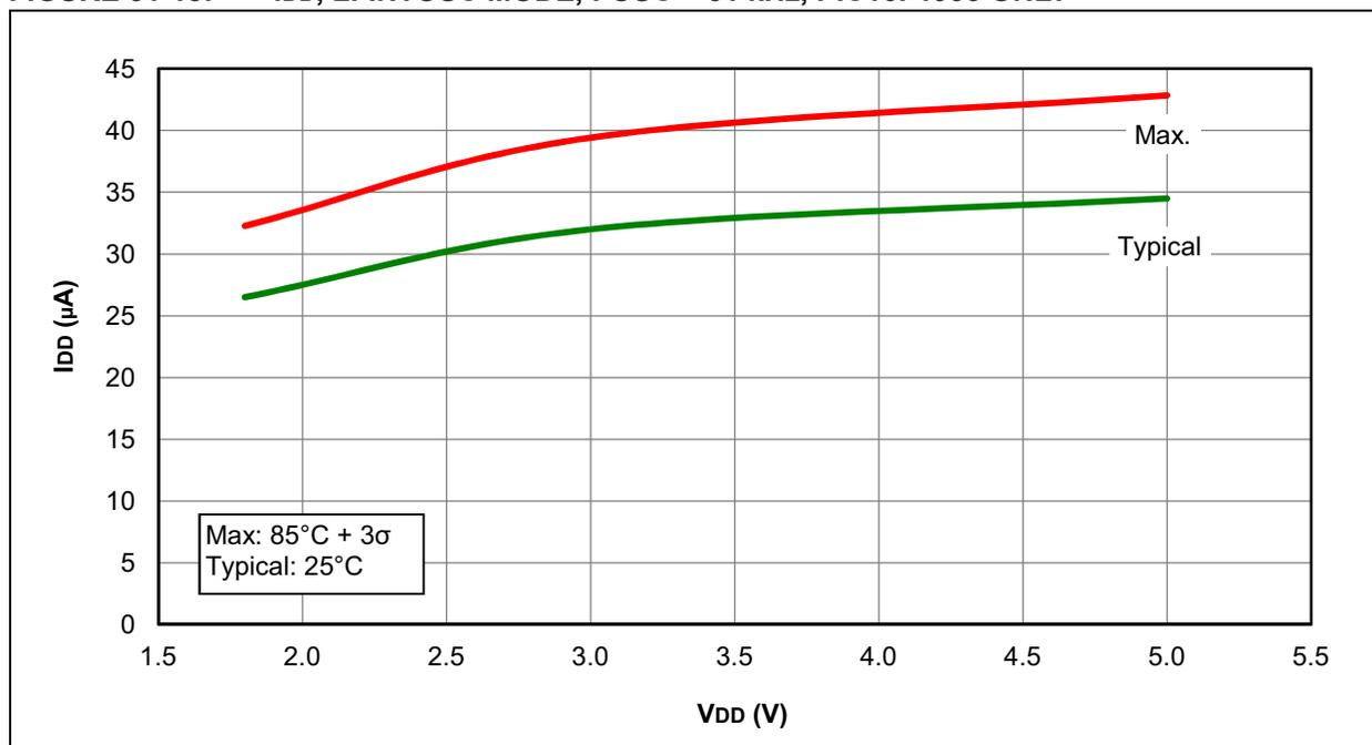
**FIGURE 31-19: I<sub>DD</sub>, MFINTOSC MODE, FOSC = 500 kHz, PIC16LF1933 ONLY**
