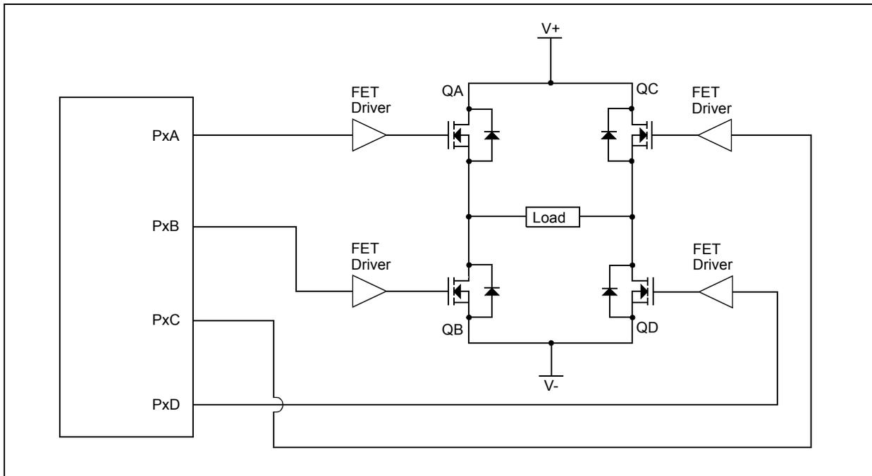
**FIGURE 23-11: EXAMPLE OF FULL-BRIDGE PWM OUTPUT**
