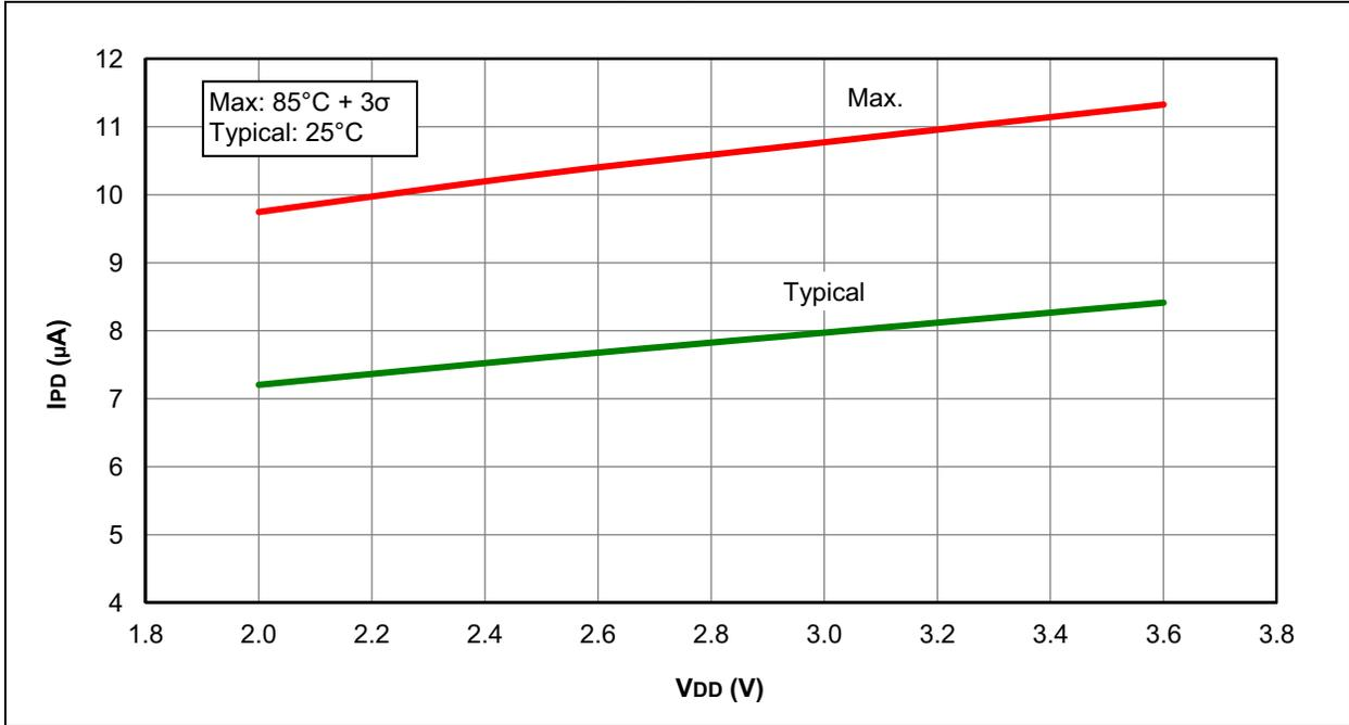
**FIGURE 31-36: I<sub>PD</sub>, BROWN-OUT RESET (BOR), PIC16F1933 ONLY**
