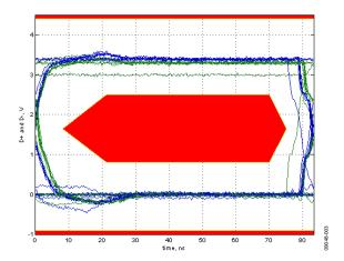
Figure 3. Full Speed Eye Diagram Showing Exclusion Zone
