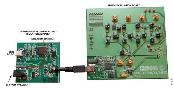
Figure 4. Photo of ADuM4160 USB Evaluation Board Connected to USB Port of AD7991 Evaluation Board
