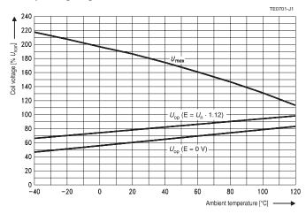
Does not take into account the temperature rise due to the contact current E=pre-energization..
