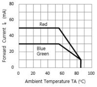
Fig. 3 FORWARD CURRENT VS. DERATING CURVE
