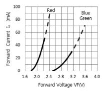
Fig. 2 FORWARD CURRENT VS. FORWARD VOLTAGE
