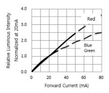
Fig. 4 RELATIVE LUMIOUS INTENSITY VS. FORWARD CURRENT
