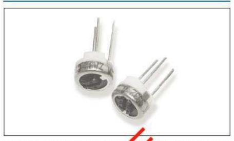
For applications that demand a durable, miniature triaming potentiometer, this military style offers quality at the right price. Cermer element technology ensures stability and performance in these 6mm diameter components. All ones are fully sealed to withstand immersion in normal board washing scients.
