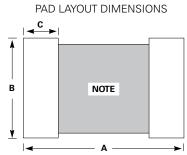
NOTE : Avoid metal runs in this area, parts not recommended for use in applications using Silver (Ag) epoxy paste.
