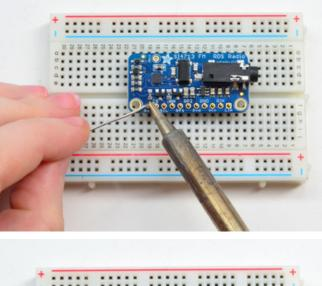
And Solder! Be sure to solder all pins for reliable electrical contact.
