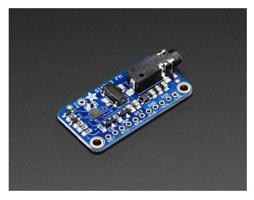
Wire up to your favorite microcontroller (we suggest an Arduino) to the I2C data lines to set the transmit frequency and play line-level audio into the stereo headphone jack. Boom! Now you **are** the media. Listen using any FM receiver such as your car or pocket radio receiver - this is an easy way to transmit audio up to about 10 meters / 30 feet away.
