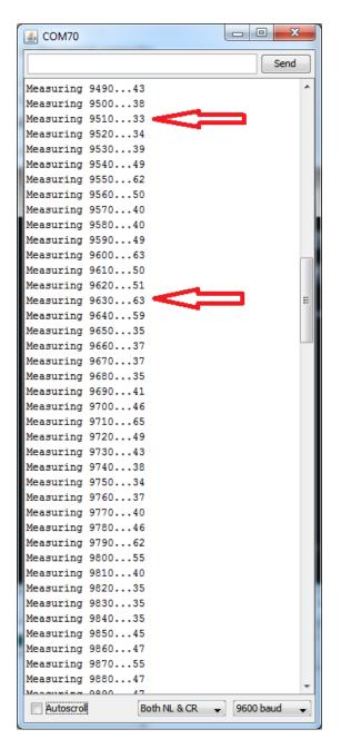
The larger the number the higher the transmission power. For example, 96.3MHz is a higher number than the others (FYI, its Univision 96.3 FM (https://adafru.it/dBs)!) whereas 95.1 MHz is nice as low, that's not used for any transmission. Try to find a number that's also not surrounded by high numbers, since it can get 'drowned out' by the nearby frequencies.
