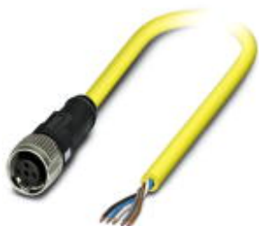
Sensor/actuator cable, 5-position, PVC, yellow, free cable end, on Socket straight M12 SPEEDCON, coding: A, cable length: 2 m
