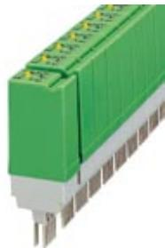
Relay connector, fitted with miniature switching relay, contacts (AgNi): Medium to large loads, 1 PDT, 230 V AC input voltage, with light indicator, can be plugged into basic terminal blocks
