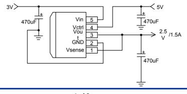
1.5A ULTRA LOW DROPOUT POSITIVE ADJUSTABLE OR FIXED-MODE REGULATOR
