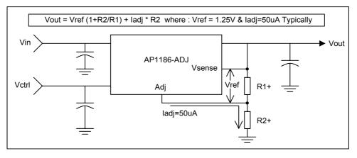
The AP1186-ADJ keeps a constant 1.25V between the Vsense pin and the Adj pin. By placing a resistor R1 across these two pins and connecting the Vsense and Vout pin together, a constant current flows through R1, adding to the ladj current and into the R2 resistor producing a voltage equal to the (1.25/R1)\*R2 + ladj\*R2. This voltage is then added to the 1.25V to set the output voltage. This is summarized in the above equation.
