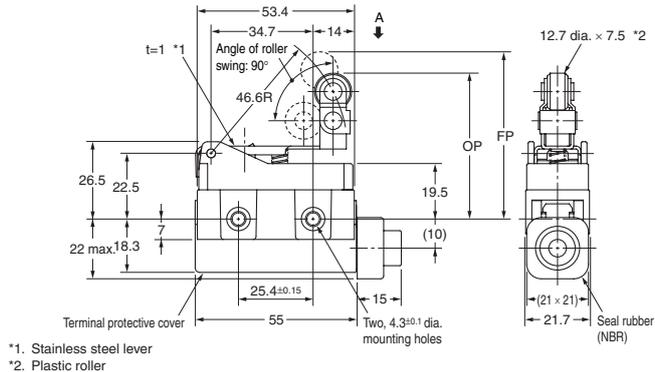
Note: 1. Unless otherwise specified, a tolerance of ±0.4 mm applies to all dimensions.
