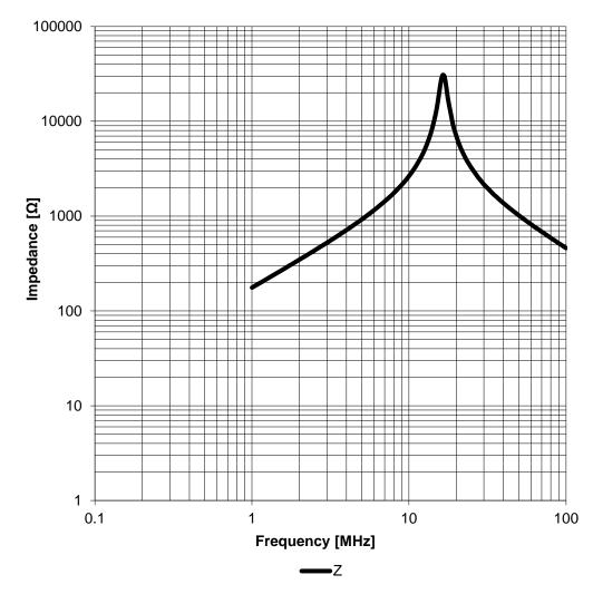
GENERAL TOLERANCE PROJECTION METHOD CREATED CHECKED Würth Elektronik eiSos GmbH & Co. KG **EMC & Inductive Solutions** KaS ChriB DIN ISO 2768-1m Max-Eyth-Str. 1 74638 Waldenburg **WE-LQS SMT Power Inductor** Tel. +49 (0) 79 42 945 - 0 ORDER CODE www.we-online.com 74404063330 eiSos@we-online.com DATE (YYYY-MM-DD) BUSINESS UNIT REVISION PAGE 001.004 2018-09-24 2/6 Valid WÜRTH ELEKTRONIK
