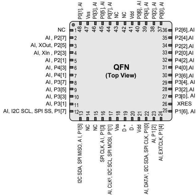
LEGEND A = Analog, I = Input, O = Output, NC = No Connection H = 5 mA High Output Drive, R = Regulated Output.
