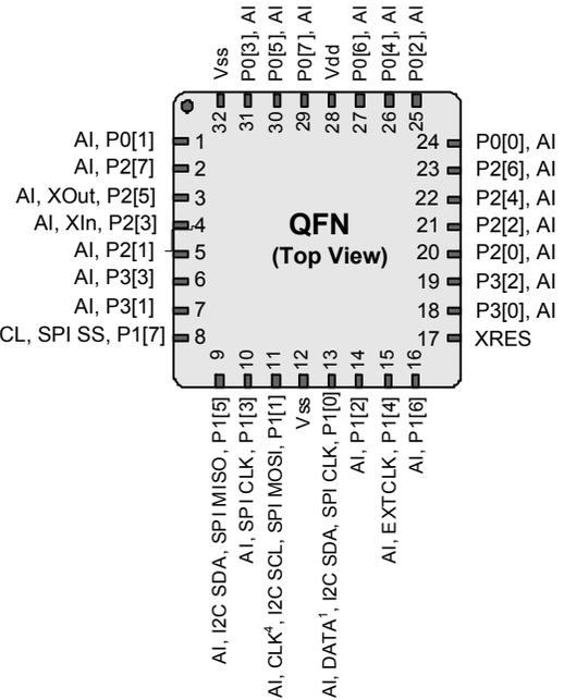
LEGEND A = Analog, I = Input, O = Output, OH = 5 mA High Output Drive, R = Regulated Output.
