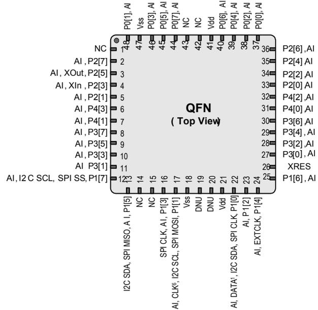
LEGEND A = Analog, I = Input, O = Output, NC = No Connection H = 5 mA High Output Drive, R = Regulated Output.
