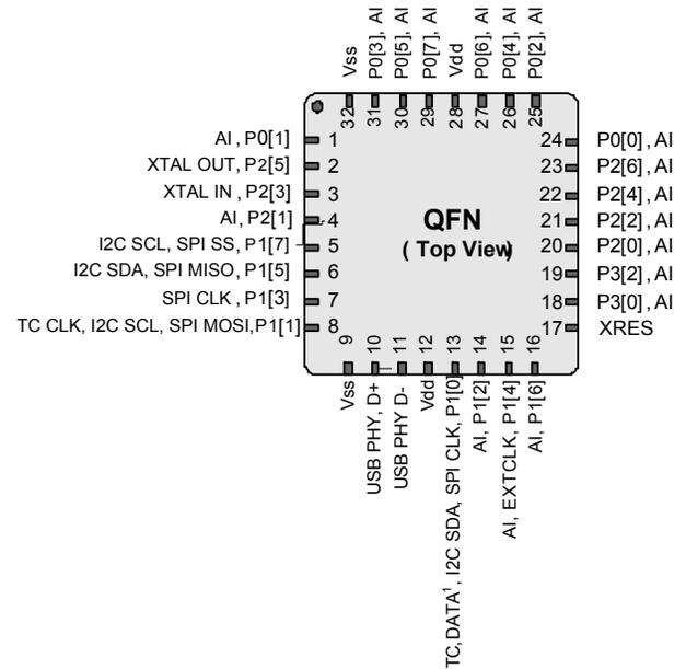
LEGEND A = Analog, I = Input, O = Output, OH = 5 mA High Output Drive, R = Regulated Output.
