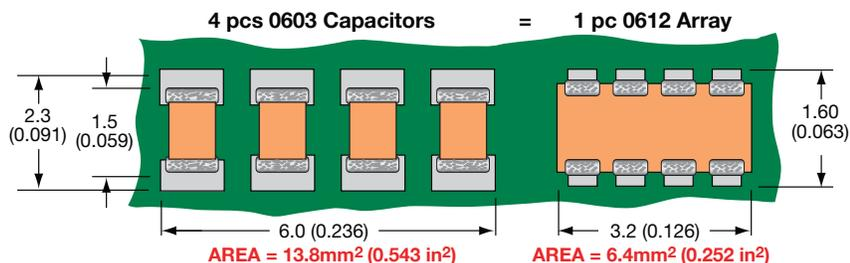
The 0612 4-element capacitor array gives a PCB space saving of over 50% vs four 0603 discrettes and over 70% vs four 0805 discrete capacitors.
