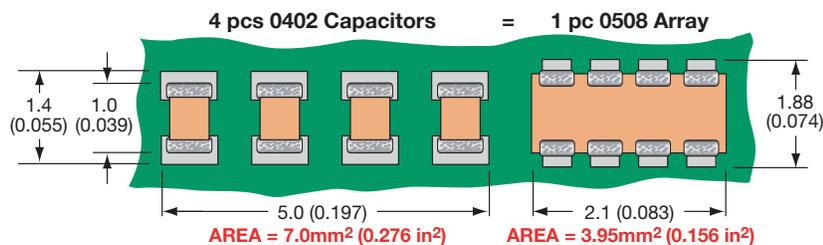
The 0508 4-element capacitor array gives a PCB space saving of over 40% vs four 0402 discrettes and over 70% vs four 0603 discrete capacitors.
