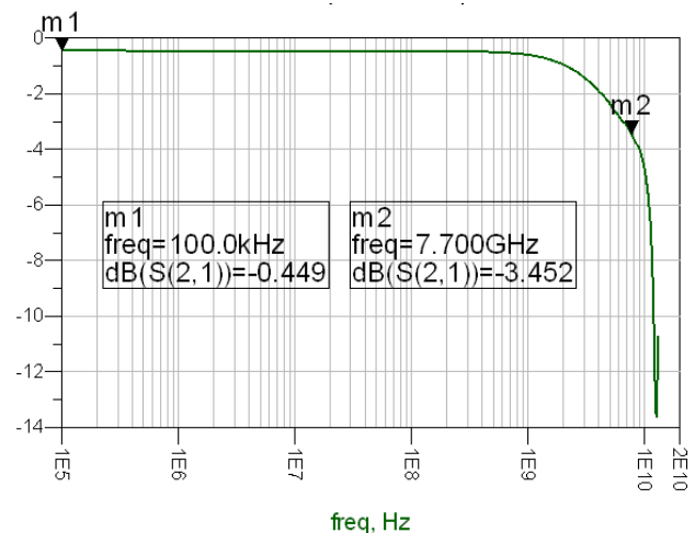
Figure 4. Bandwidth for USB Switch
