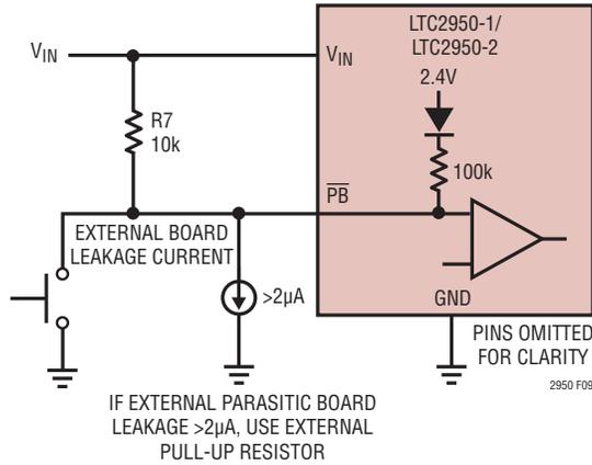
Figure 9. External Pull-Up Resistor on  $\overline{PB}$  Pin
