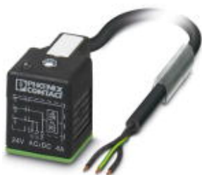
Sensor/actuator cable, 3-position, PUR/PVC, black RAL 9005, free cable end, on Valve connector A, with 1 LED, connected with Z diode, cable length: 1.5 m
