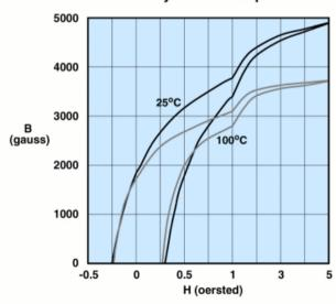
Measured on an 18/10/6mm toroid at 10kHz.
