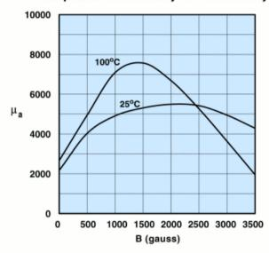
Measured on an 18/10/6mm toroid at 10kHz.
