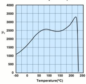
Measured on an 18/10/6mm toroid at 100kHz.
