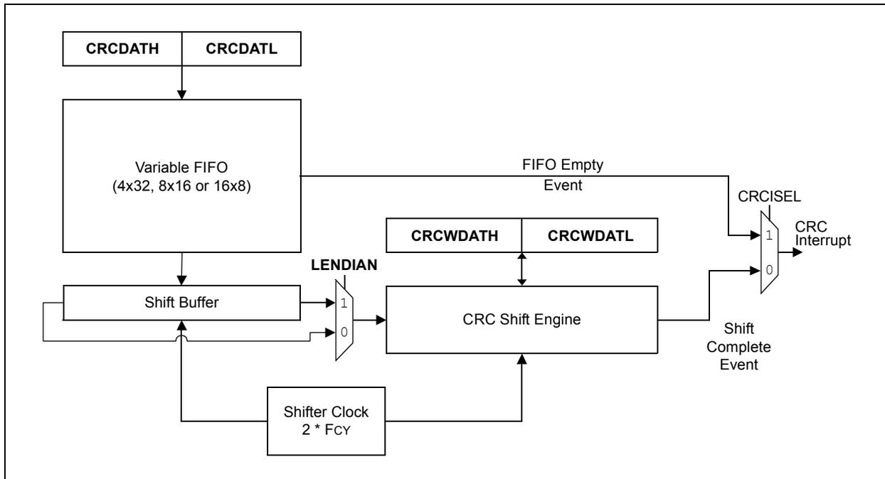
FIGURE 23-2: CRC SHIFT ENGINE DETAIL
