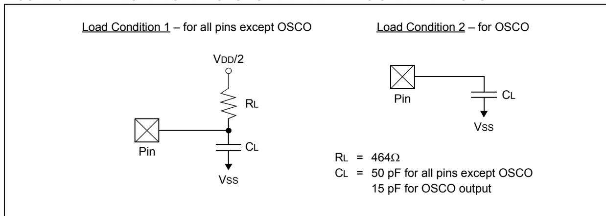
**TABLE 32-18: CAPACITIVE LOADING REQUIREMENTS ON OUTPUT PINS**
