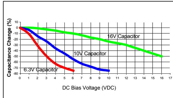
When selecting a ceramic capacitor to be used with the internal voltage regulator, it is suggested to select a high-voltage rating, so that the operating voltage is a small percentage of the maximum rated capacitor voltage. For example, choose a ceramic capacitor rated at 16V for the 2.5V or 1.8V core voltage. Suggested capacitors are shown in [Table 2-1](#).
