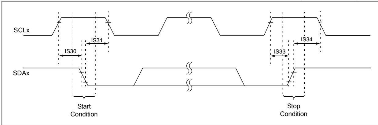
**TABLE 32-24: I<sup>2</sup>C™ BUS START/STOP BIT TIMING REQUIREMENTS (SLAVE MODE)**
