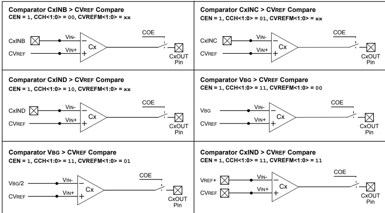
**FIGURE 25-4: INDIVIDUAL COMPARATOR CONFIGURATIONS WHEN CREF = 1 AND CVREFP = 1**
