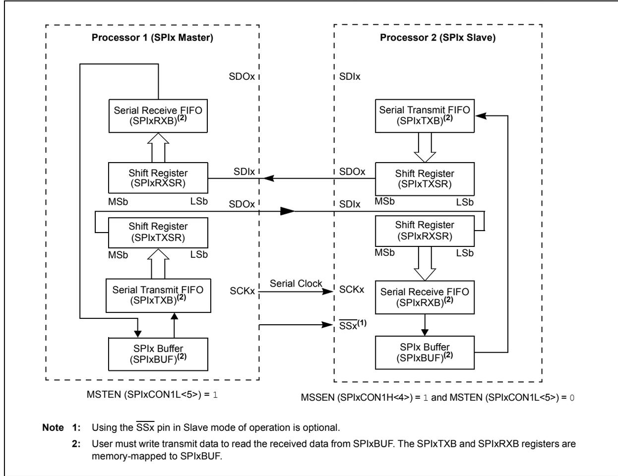
**FIGURE 16-5: SPIx MASTER, FRAME MASTER CONNECTION DIAGRAM**
