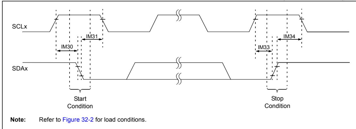
**TABLE 32-22: I<sup>2</sup>C™ BUS START/STOP BIT TIMING REQUIREMENTS (MASTER MODE)**
