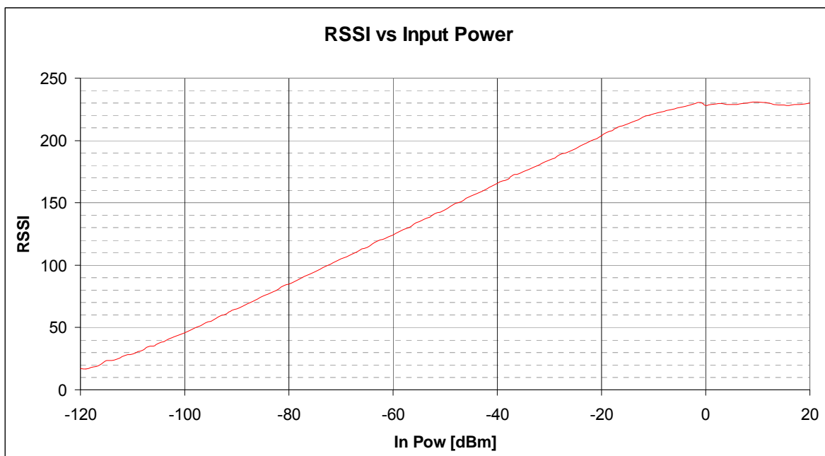
Figure 23. RSSI Value vs. Input Power
