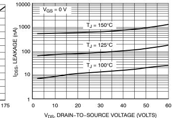
Figure 6. Drain-to-Source Leakage Current versus Voltage
