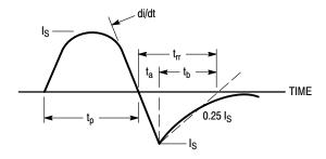
Figure 14. Diode Reverse Recovery Waveform
