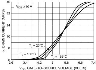
Figure 2. Transfer Characteristics
