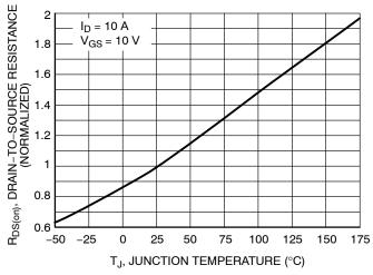
Figure 5. On-Resistance Variation with **Temperature**
