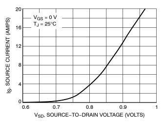
Figure 10. Diode Forward Voltage versus Current
