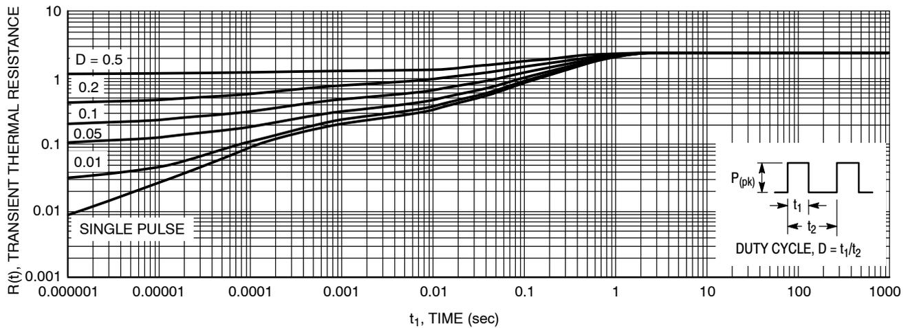
**Figure 10. Thermal Response Junction-to-Case for MBRF30H60CTG and MBRJ30H60CTG**
