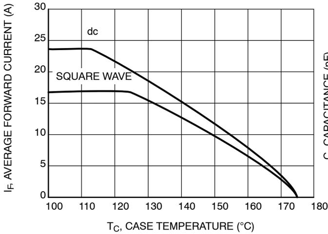
**Figure 8. Current Derating for MBRF30H60CTG and MBRJ30H60CTG**
