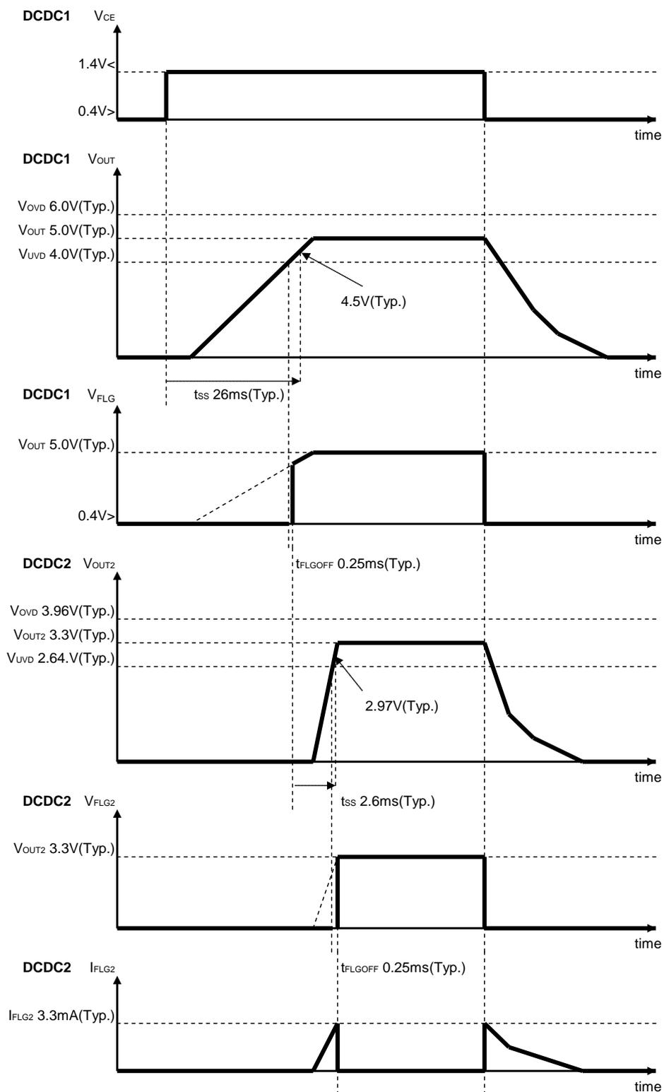
Fig. 3 Start-up/ Shutdown Sequencing
