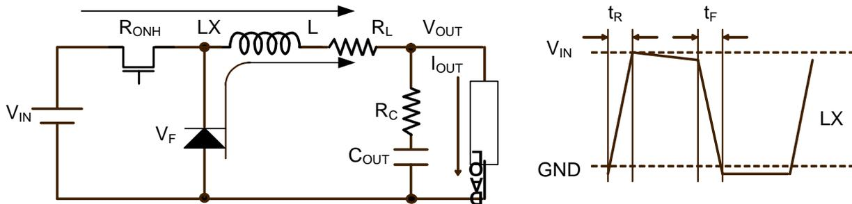
Nch High-side Tr. Turn-on Loss:  $P_{ON} = R_{ONH} \times I_{OUT}^2 \times \text{Onduty}$
