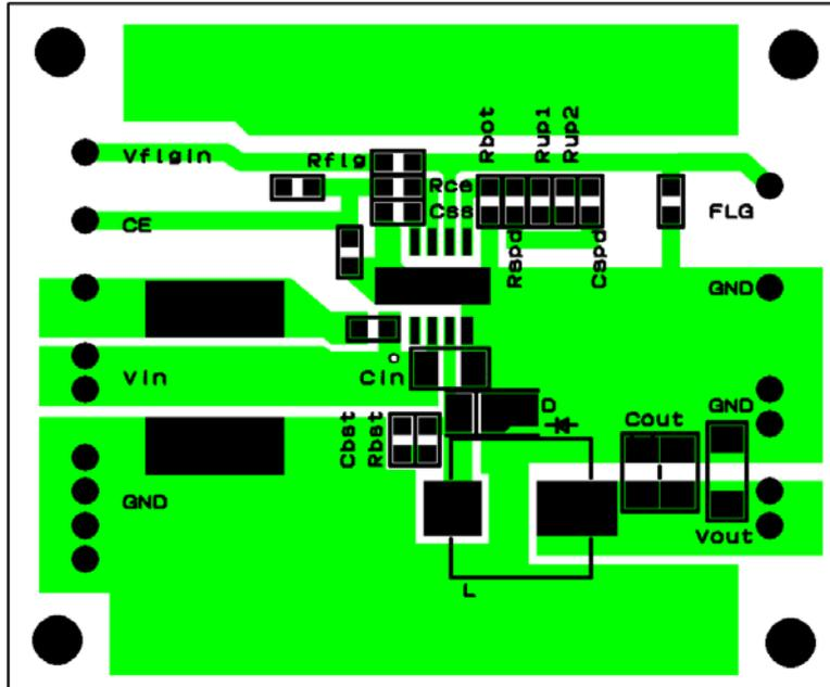
(The broad land of Lx section enables a connection with large inductors and diodes).
