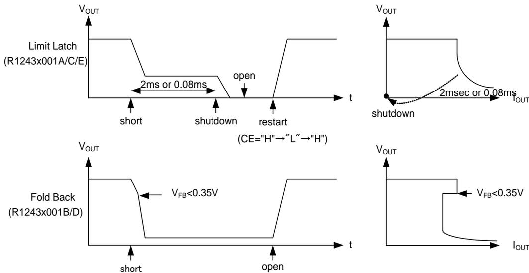
**Fig. 5 LX Current Limit Sequencing**
