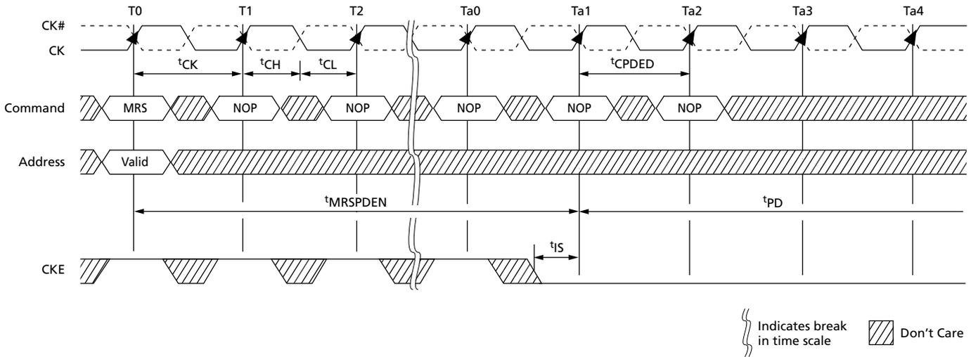
**Figure 105: Power-Down Exit to Refresh to Power-Down Entry**
