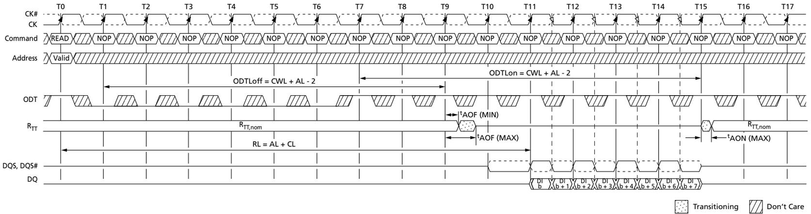
Note: 1. ODT must be disabled externally during READs by driving ODT LOW. For example, CL = 6; AL = CL - 1 = 5; RL = AL + CL = 11; CWL = 5; ODTLon = CWL + AL - 2 = 8; ODTLoff = CWL + AL - 2 = 8. R<sub>TT,nom</sub> is enabled. R<sub>TT(WR)</sub> is a "Don't Care."
