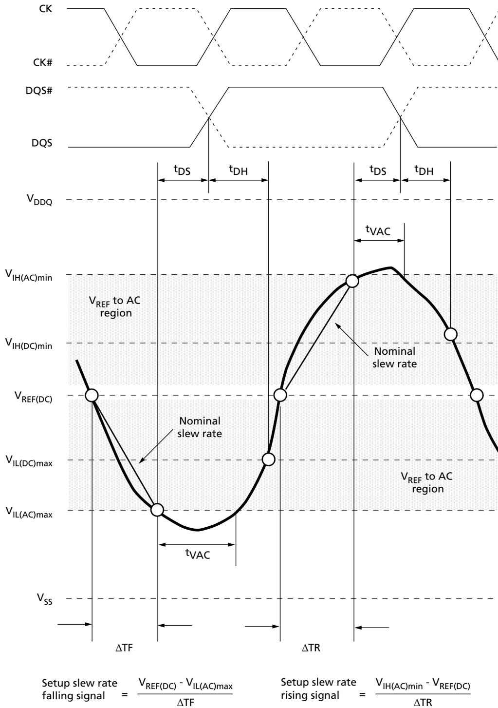
Note: 1. The clock and the strobe are drawn on different time scales.
