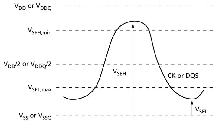
**Figure 18: Definition of Differential AC-Swing and  $t_{DVAC}$**
