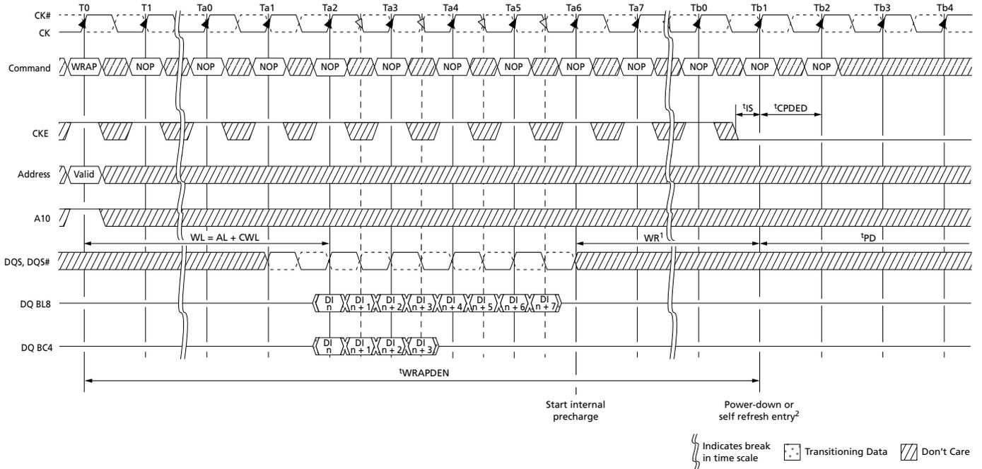
Notes: 1.  $t\text{WR}$  is programmed through MR0[11:9] and represents  $t\text{WRmin}$  (ns)/ $t\text{CK}$  rounded up to the next integer  $t\text{CK}$ .
