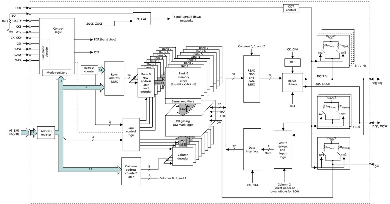
**Figure 4: 128 Meg x 8 Functional Block Diagram**
