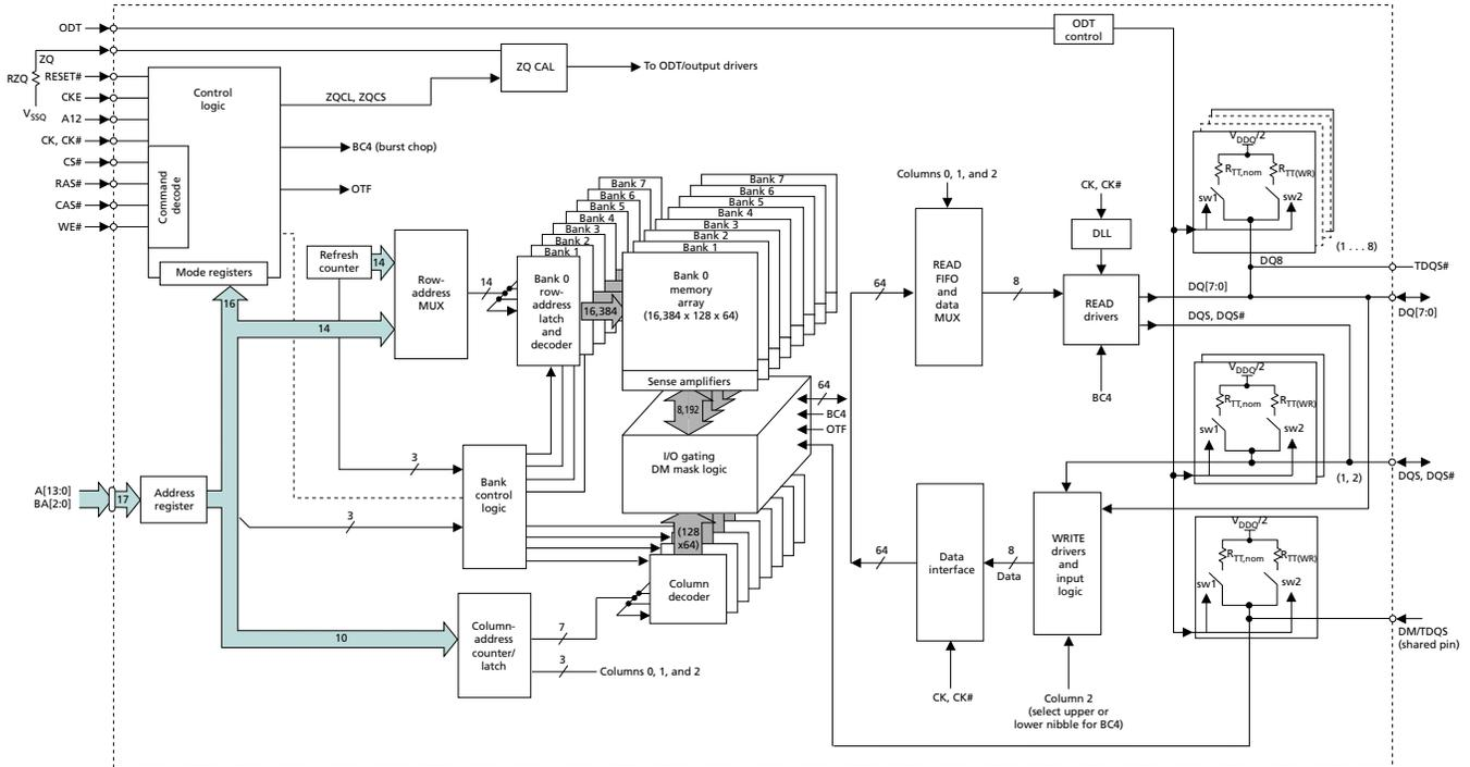
**Figure 5: 64 Meg x 16 Functional Block Diagram**
