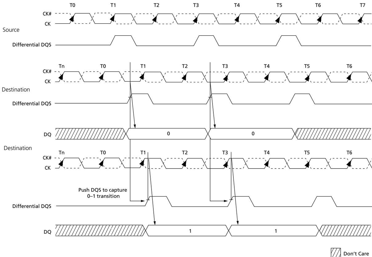
When write leveling is enabled, the rising edge of DQS samples CK, and the prime DQ outputs the sampled CK's status. The prime DQ for a x4 or x8 configuration is DQ0 with
