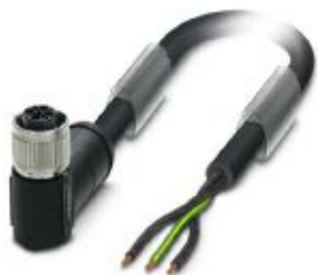
Power cable, 3-position, PVC, black, free cable end, on Socket angled M12, coding: S, cable length: 1 m, for AC current up to 16 A/230 V
