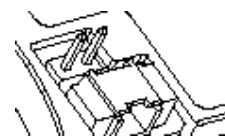
Figure 9: Master Setting for Vertical iDiskOnChip 40-Pin Connector
