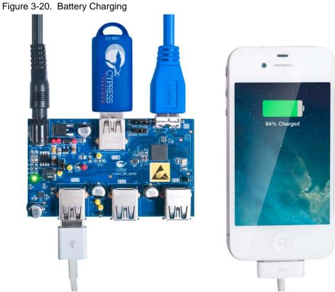
Note: For the CY4613 kit, battery charging is supported only on standard USB 3.0 ports and Shared Link USB 2.0 ports. Battery charging is not supported on Shared Link SS ports because the SS ports are expected to be embedded ports and not exposed.
