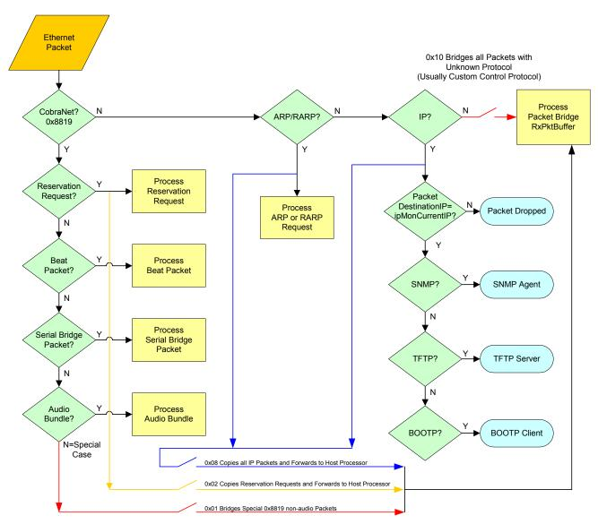
Figure 4. Packet Bridge Receive Filtering
