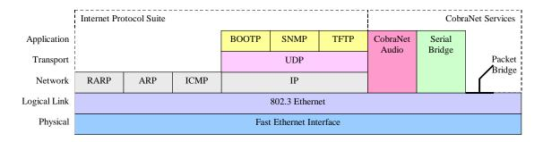
Figure 5. CobraNet Network Stack
