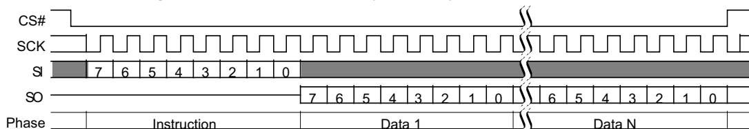
Figure 48. Read Identification (RDID 9Fh) Command Sequence
