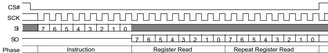
Figure 54. Read Bank Register (BRRD 16h) Command
